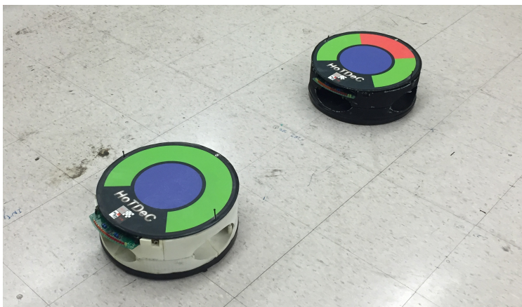
Figure 5.1: Experimental setup of the hovercrafts. The white vehicle is following a circular trajectory while the black vehicle is trying to follow it.
