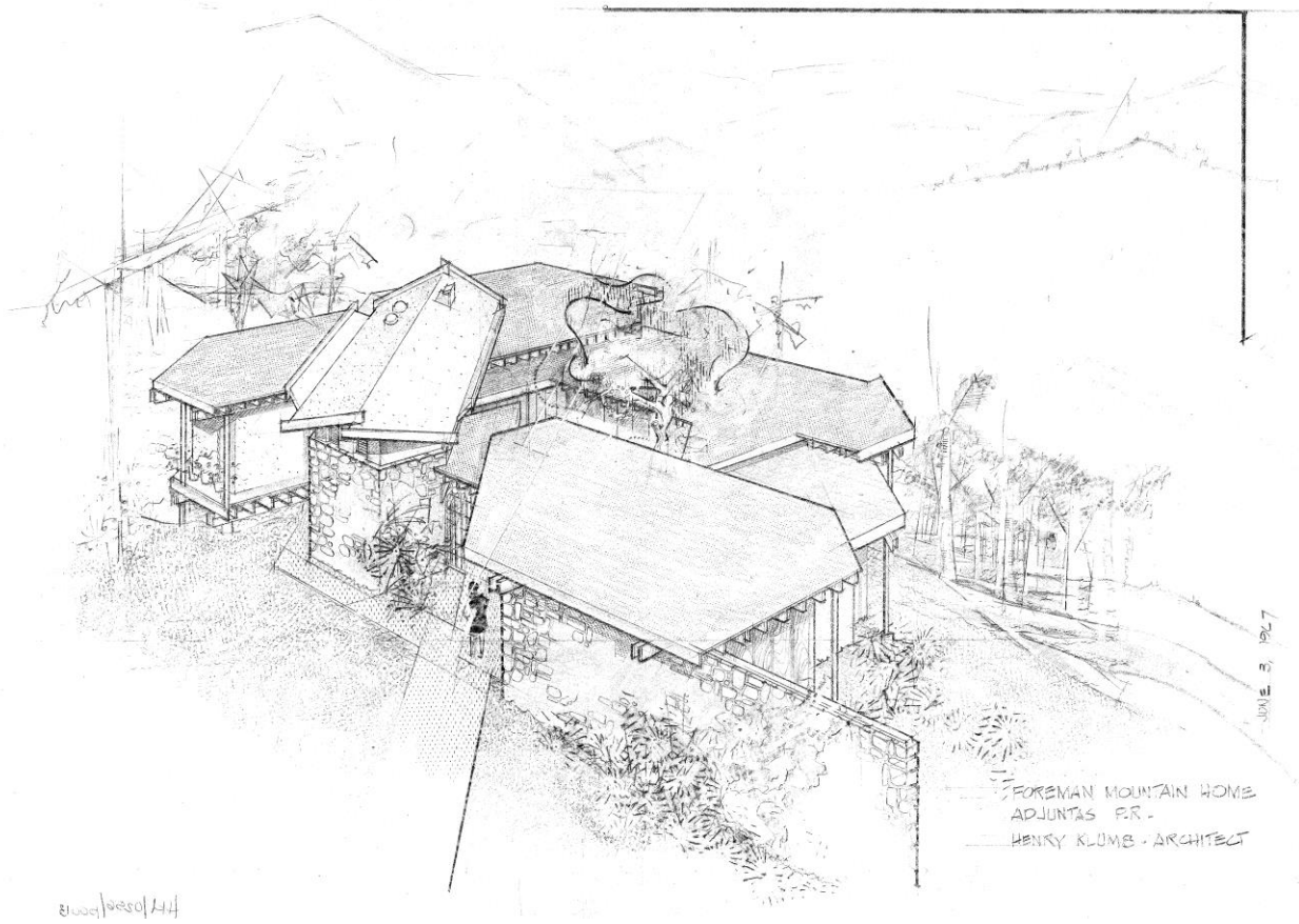
Figure 4.20. Aerial perspective, the Foreman Mountain Retreat. The site slopes down to the south. The two principal wings of the house are at the upper left (the long axis in the description above) and upper right in the drawing. Drawing by Henry Klumb/The Office of Henry Klumb, courtesy of the AACUPR.
