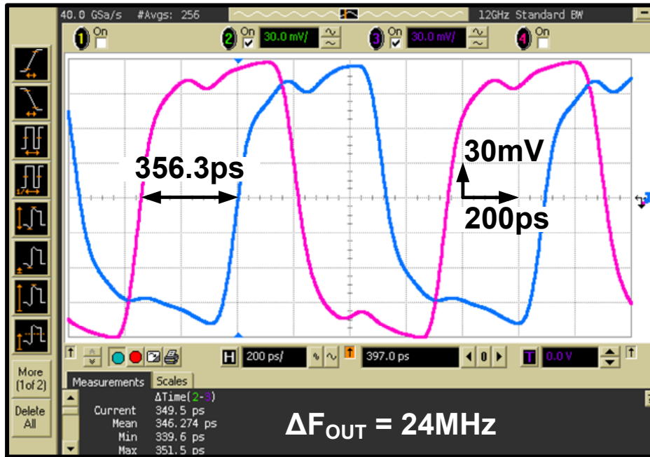
Figure 6.7: Measured CCRO IP/N time domain waveforms at frequency offset of 24 MHz.
