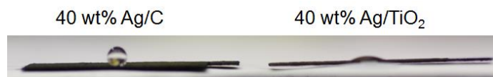
Figure 2.7 Image of wettability difference between catalyst layers of 40 wt% Ag/C and 40 wt% Ag/TiO 2 . Reprinted with permission from ChemSusChem 7, 866-874, (2014). Copyright 2013 Wiley.
