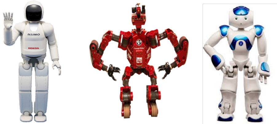
(a) Examples of statically stable biped robots: ASIMO (left), CHIMP (middle) and NAO (right). For these robots, stability can be achieved while keeping a particular posture.
