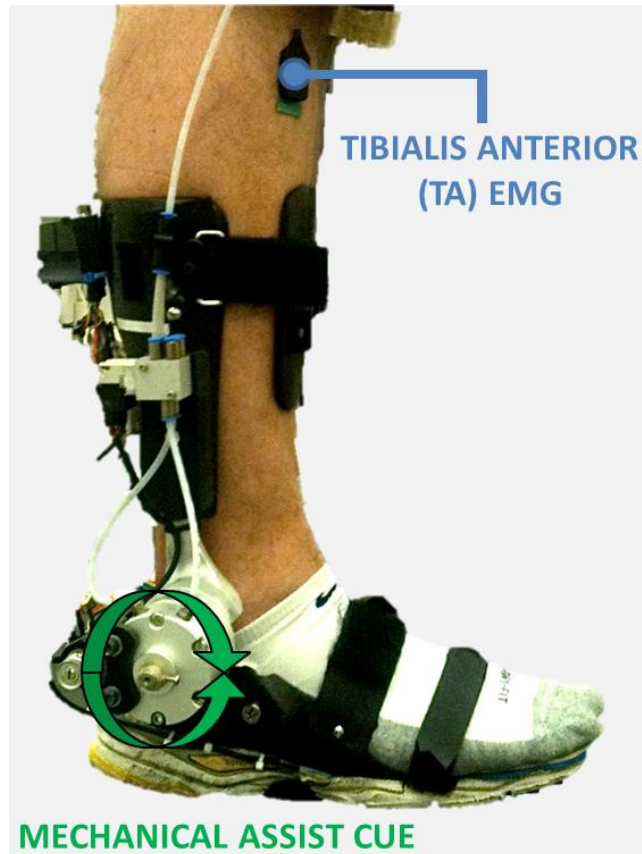
Figure 6: Experimental set up with the PPAFO attached to the right leg. Ground reaction force (GRF) data were recorded from two force plates under each foot. Bipolar surface EMG signals were recorded from an electrode placed over the right tibialis anterior (TA).
