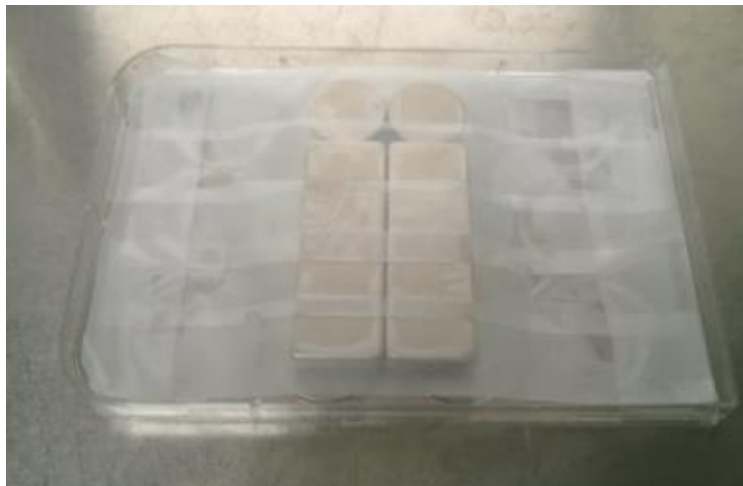
Figure 5.9 Permanent rare earth magnets taped to the underside of a well plate cover. Well plates with samples inside them can be placed on top of this well plate cover to introduce a magnetic field.
