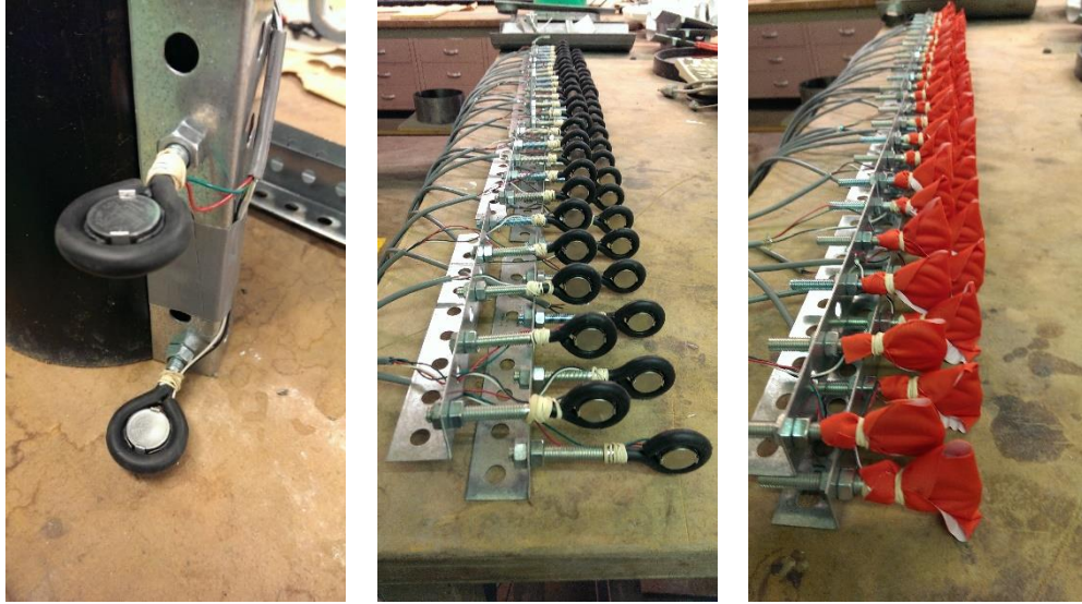
Figure 2-3 Construction of iButton sensors (left), fitted with rubber bands (center), and covered in GORE-TEX fabric (right).
