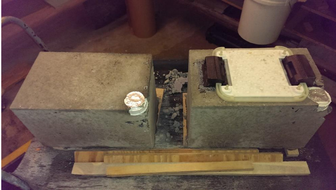
Figure 3-12 De-molded model concrete crossties with PVC access plug where multi-conductor shielded cables are encase.
