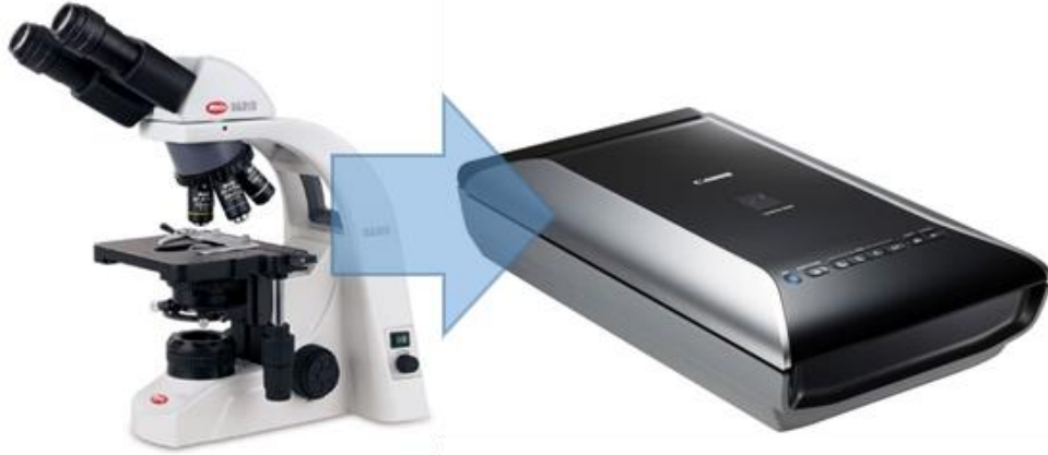
Figure 7-1 Optical microscope conventionally used in ASTM C457 to measure air-void parameters is replaced with a high-resolution flatbed scanner in order to draw the same information from a 2-dimensional scanned image.
