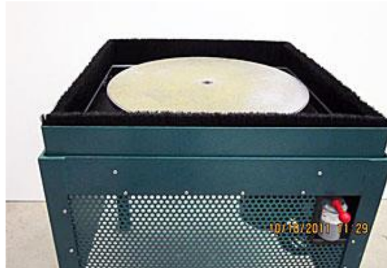
Figure 7-6 Forty-five cm (18 inch) diameter grinding wheel used to polished hardened concrete sections (from ASW Diamond).
