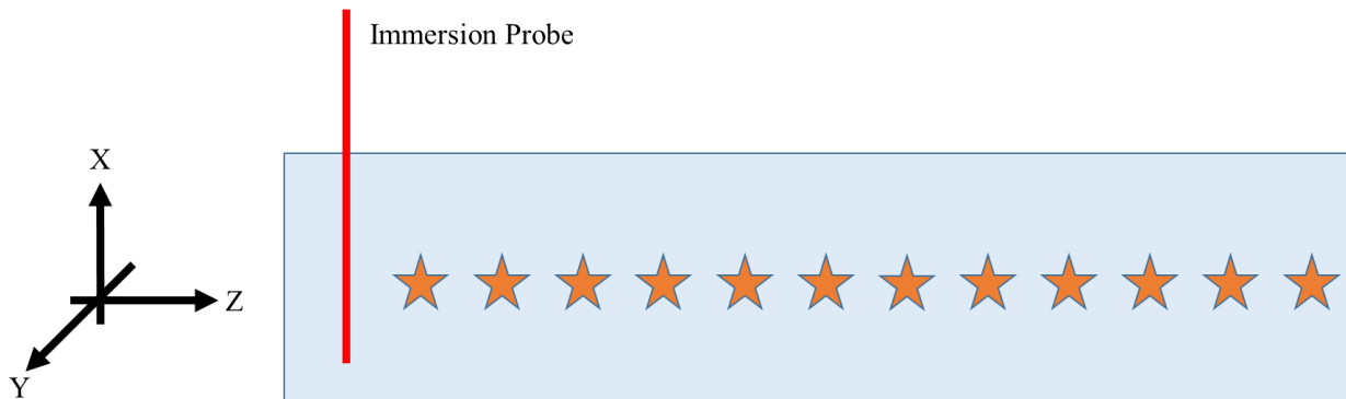
Figure 6-4 Illustration of immersion pencil (probe) vibrator in 48-inch long Plexiglas mold where stars represent the nominal location of an immersed accelerometer spaced 1 or 2 inches apart during vibratory testing.
