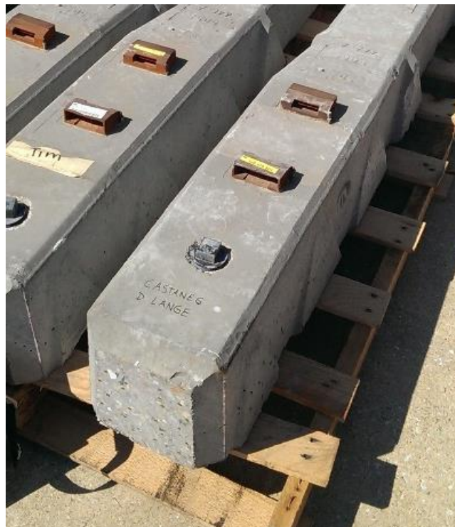
Figure 2-6 De-molded concrete crossties with square cap added to PVC access plug where multi-conductor shielded cables are encased.
