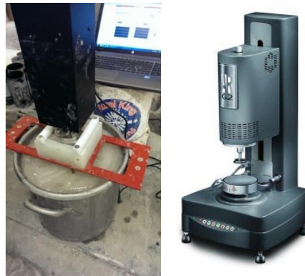
Figure 5-2 An ICAR concrete rheometer (left) with Carbopol-mortar and an AR-G2 high-precision rheometer (right).
