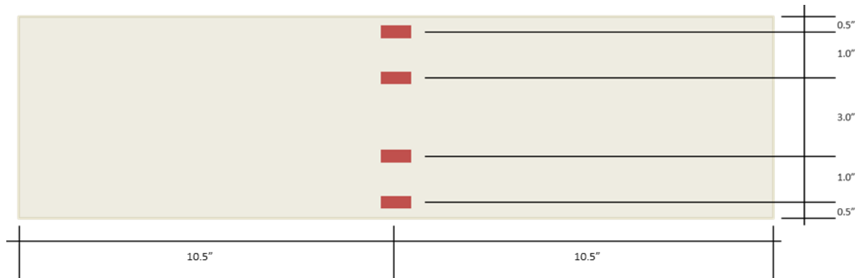
Figure 2-10 Illustration of 6 x 6 x 21 inch modulus of rupture concrete beam instrumented with hydrochron sensors at depths of 0.5, 1.5, 4.5, and 5.5 inches from the top surface. The sensors are centrally situated in the beam 3 inches from the width of the beam at 10.5 inches from either end. The beams are installed in model ballast in Rantoul, IL.
