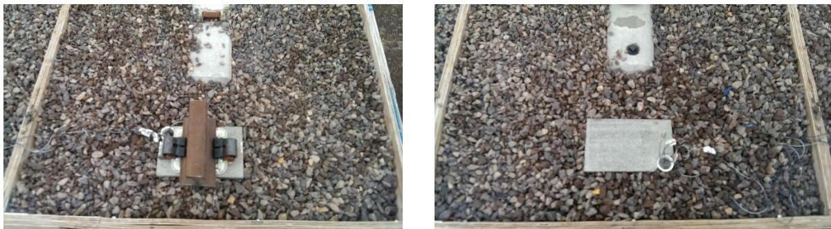
Figure 3-13 Model crossties installed in model ballast in Rantoul, IL. A polyurethane pad and steel rail section is added to the model crosstie with embedded anchors.
