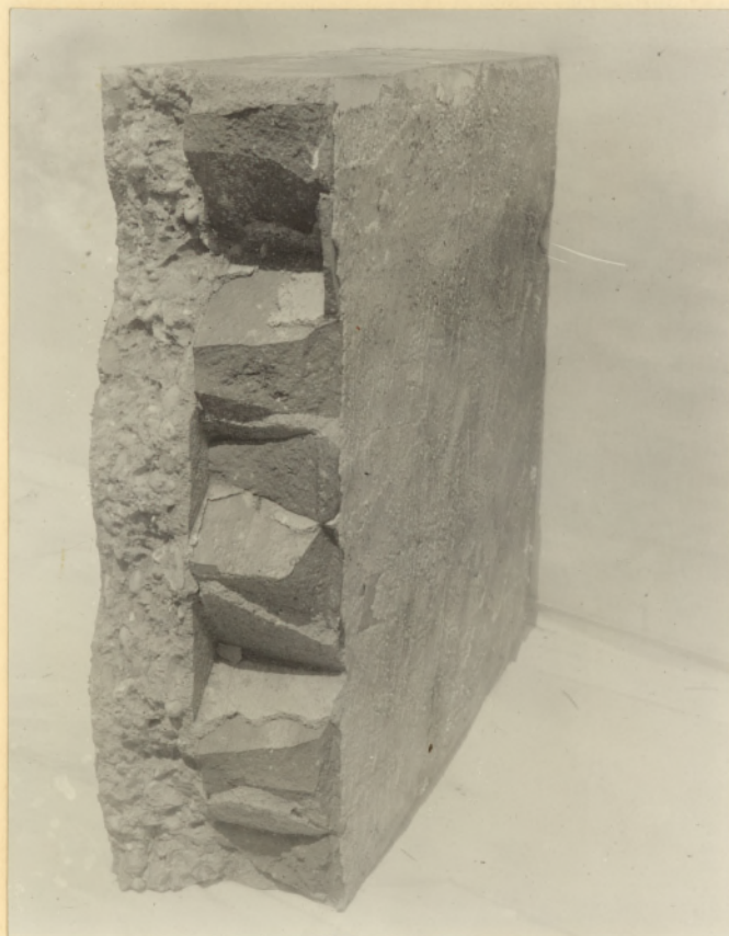
Dry mix type 4-inch brick 3-inch concrete
