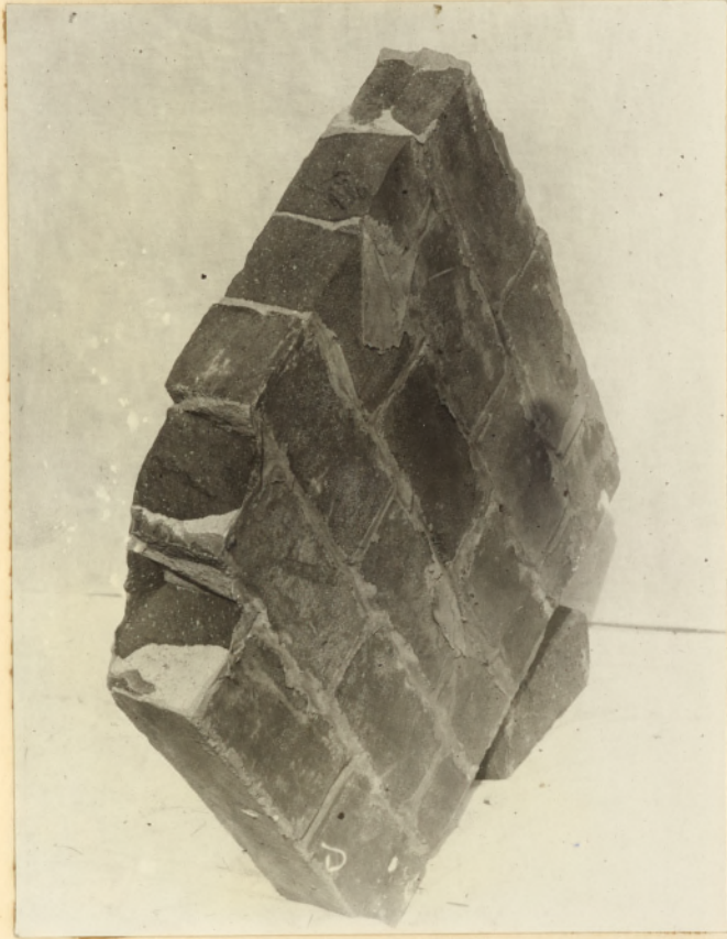
4-inch brick laid on third points
