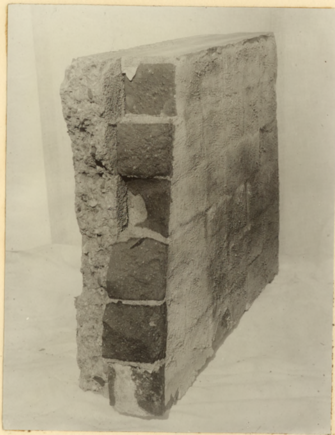
Dry mix type 4-inch brick 3-inch concrete
