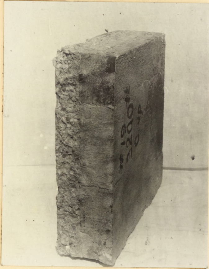
Dry mix type 4-inch brick 3-inches concrete
