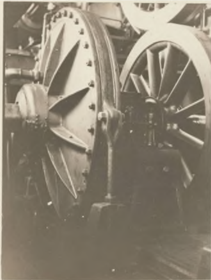
Fig. 5. Brake and Supporting Wheel, Purdue Plant.
