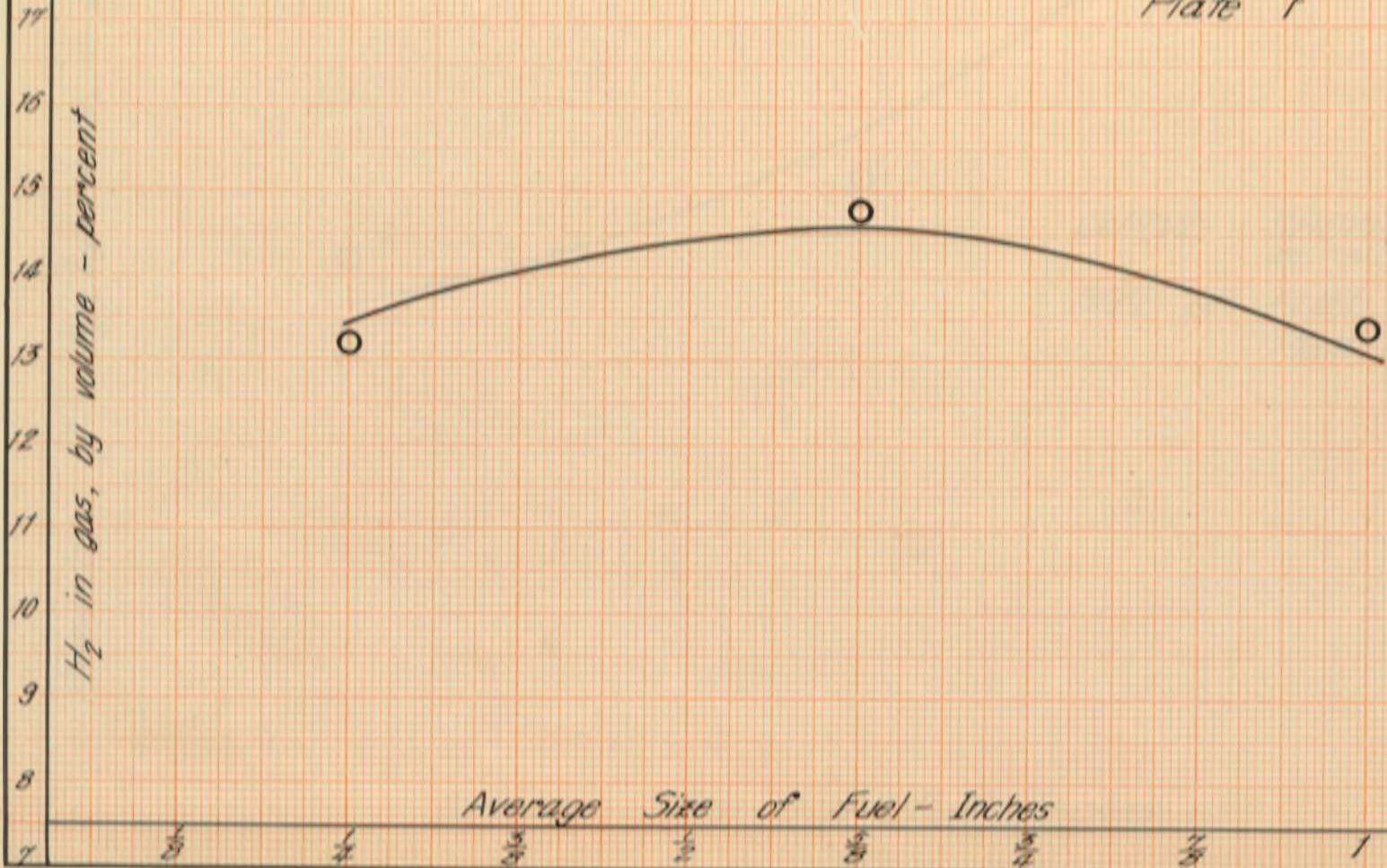
CURVE SHOWING RELATION BETWEEN SIZE OF FUEL & H 2 IN GAS Plate F
