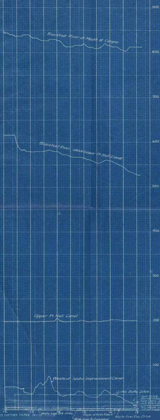
HYDROGRAPHS SHOWING DISCHARGE AT RIVER AND CANAL GAGING STATIONS MAINTAINED DURING BLACKFOOT SEEPAGE INVESTIGATION JUNE 12-17 1915
