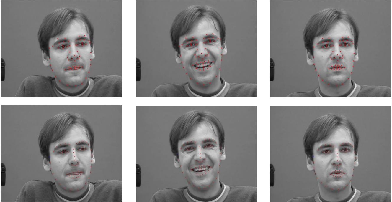
Figure 4 Top: Annotated points generated by AAM from given data set. Bottom: Annotated points produced from C2F-DPM method. Both methods produce similar points for mouth area and jawline region.
