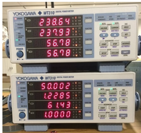
Figure 6.2: Measurements through YOKOGAWA WT310 Digital Power Meter at 50 V DC input
