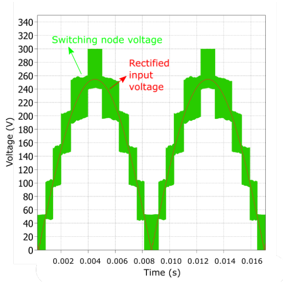
Figure 2.2: Simulated switching node voltage and rectified input voltage of the proposed FCML converter
