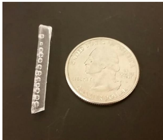
Fig. 2.8: A finished leptosporangium replica, after the water has evaporated from the droplets. A U.S. quarter is used for scale.
