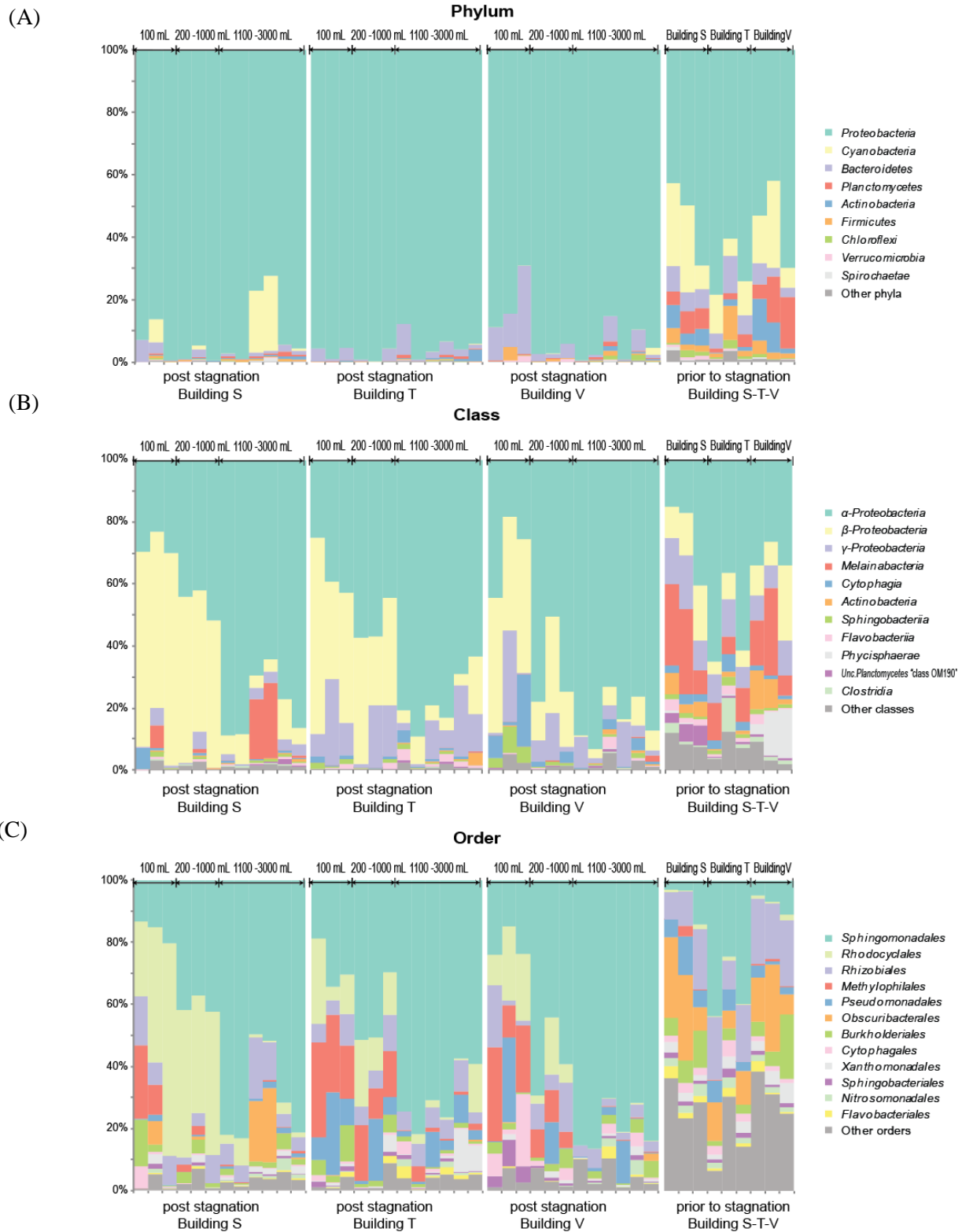
Figure 3.5 Community composition comparison between post-stagnation and pre-stagnation samples. Phyla over 0.1% (A) and classes (B) and orders (C) over 1% are shown.
