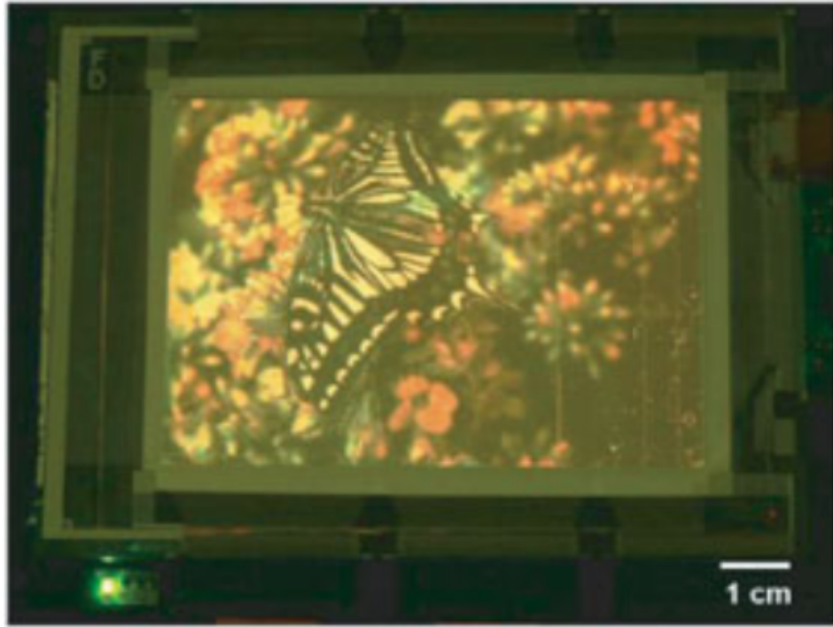
Figure 1.4: A QD display image over a thin film transistor backplane with 320x240 pixels [67].
