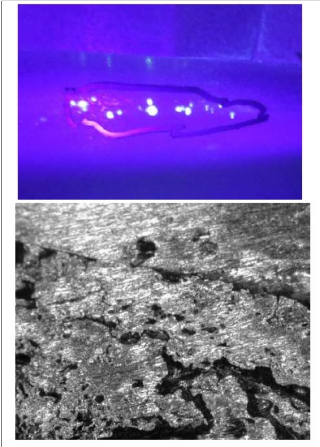
Figure 3.3: An example of circumferentially oriented point indications of arc damage on a retaining ring shrink seat as seen during a fluorescent dye inspection and one of the point locations as seen by a low-power digital microscope. As the arcing occurred between two surfaces in close contact, the arcing is level with the adjacent surface of the retaining ring [3].
