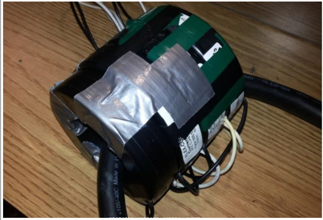
Figure 4.9: Current transformer made by connecting 4 7RL-162 1600:5 45VA CTs in series.
