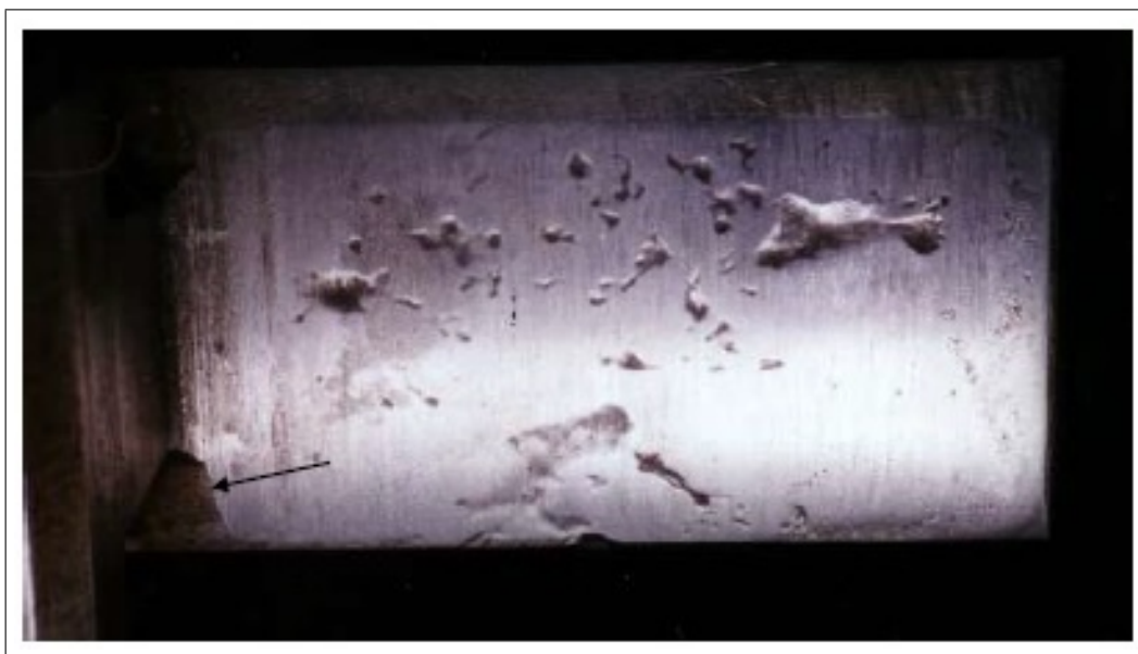
Figure 1.4: Arcing marks on rotor teeth [3].
