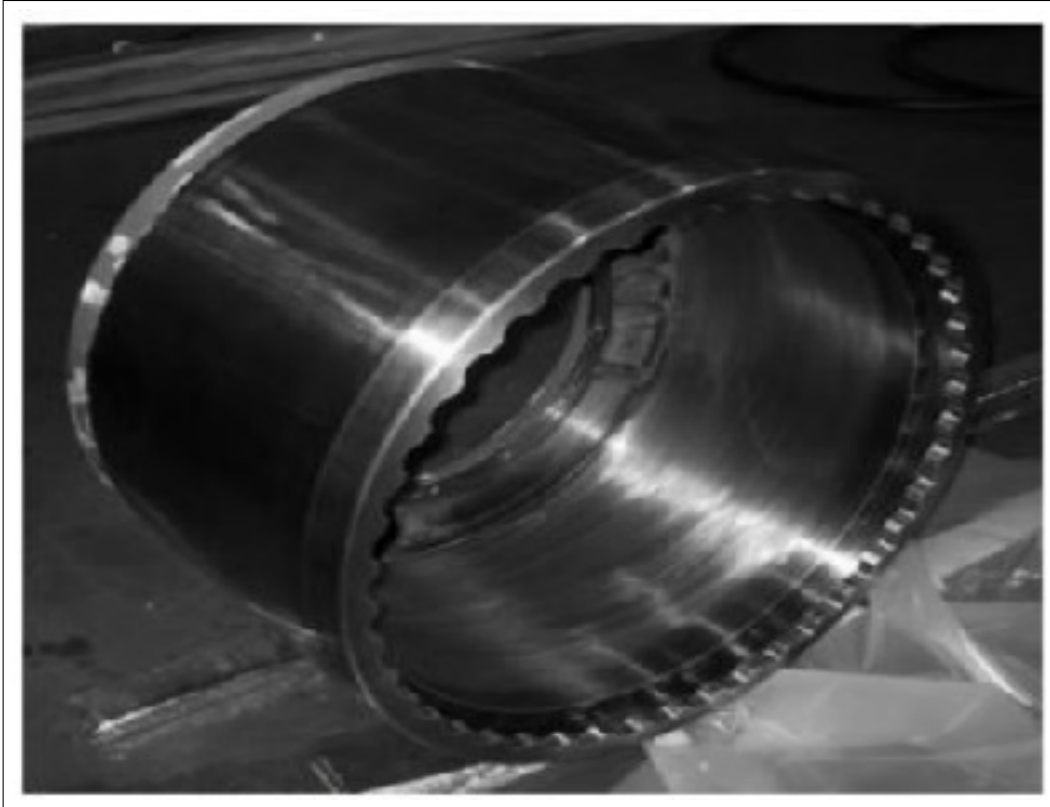
Figure 1.1: Image of retaining ring with castellations for axial restraint. [1]
