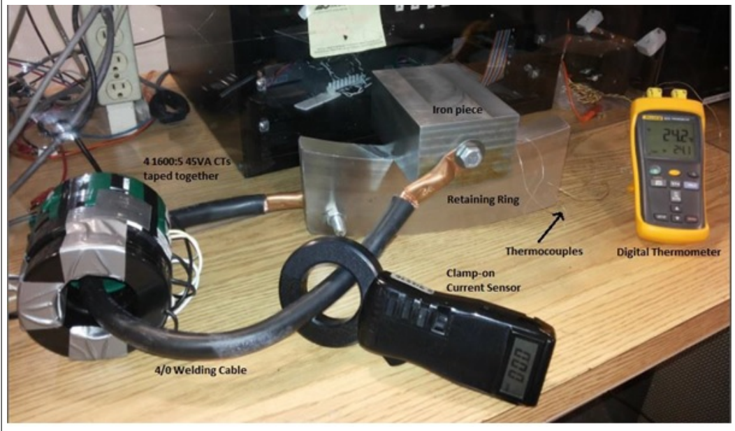
Figure 4.6: Experiment setup without compressive test machine.
