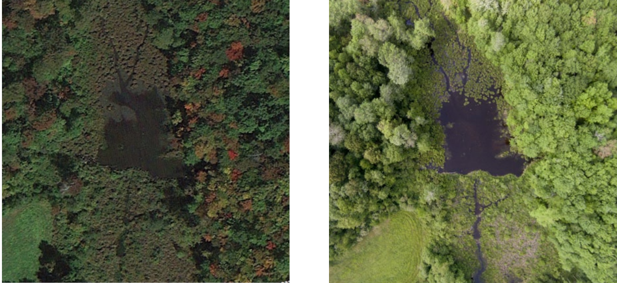
Figure 8.3 A comparison of two aerial images of a wetland: a satellite image from Google Earth at maximum zoom (left) and an image taken at an elevation of 500 feet by the author with a sUAS (right). Neither image was edited.
