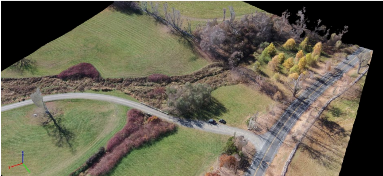
Figure 8.4 A 3D point cloud model generated with Pix4D Mapper using imagery obtained by a sUAS at an elevation of 100 feet. Imagery and model by author.
