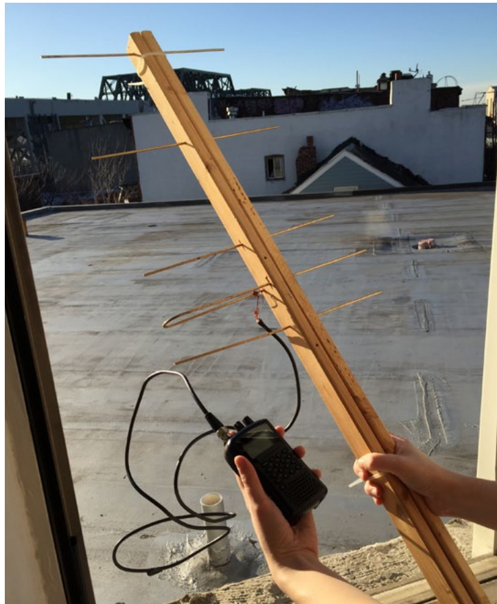
Figure 7.1 A yagi antenna created by the author.
