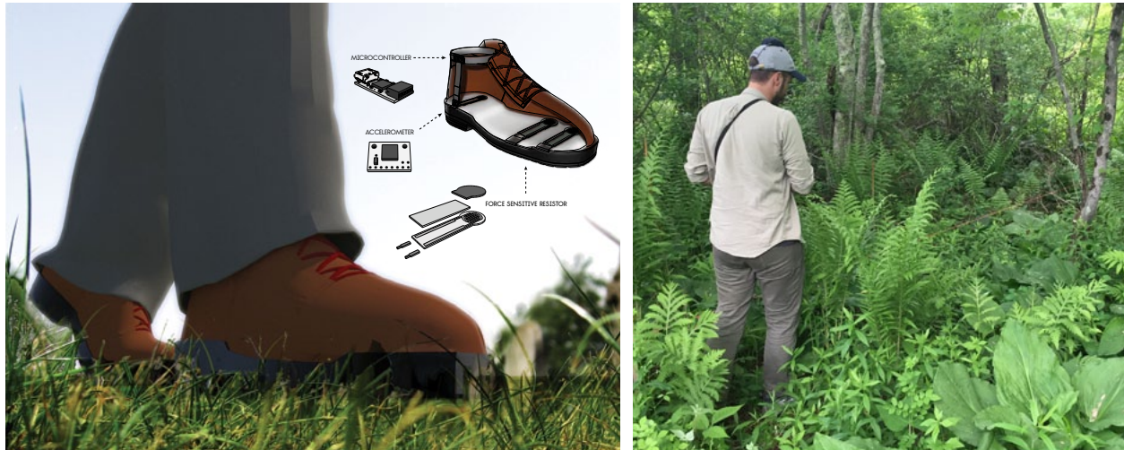
Figure 8.8 Original concept diagram of the Haptic Surveyor (left). Author testing a similar apparatus in field with a GPS antenna attached to a hat. Images by author.
