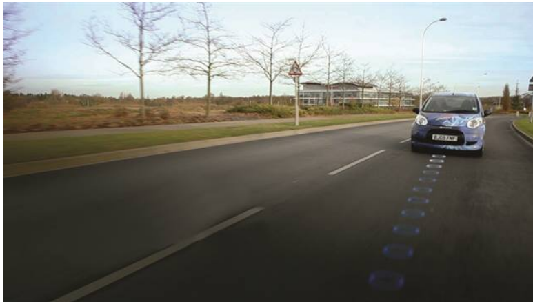
(b) Illustration of dynamic wireless charging [21].
