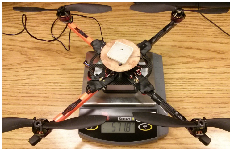
Figure 2.7: Multirotor mass. A regular laboratory scale can be used to determine the all-up weight (AUW) of the airframe to be modeled.
