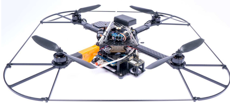
Figure 1.1: Typical example of a quadrotor UAV. Motors and propellers spaced symmetrically around the airframe's center of gravity allow the pilot to influence the aircraft's attitude and direction of travel simply by changing motor speeds between the actuators.
