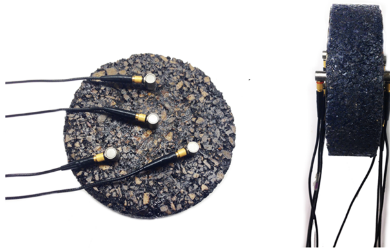
Figure 4.3: Front and side photograph of a specimen two weeks after being treated with rejuvenator with four acoustic emission sensors coupled to each of the two flat surfaces
