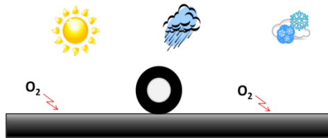
Figure 1.1: Oxidative aging of asphalt concrete pavements. With increasing oxidative aging in the top material layer, the pavement becomes increasingly more susceptible to damage accumulation due to mechanical and environmental loads.
