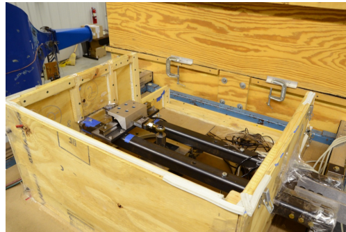
Figure 3.21: Air-tight containment box and contents located on top of wind tunnel; FPS and secondary force balance are both visible.
