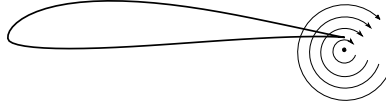
Figure 1.3: Multielement airfoil including a single element and a point vortex representing a slotted flap.
