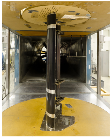
Figure 3.7: Front view of MFFS(ns)-026 airfoil mounted for testing.
