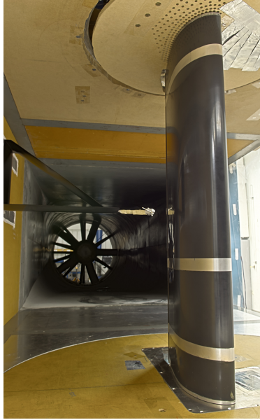
Figure 3.33: Wind tunnel model including new floor and ceiling with horizontal brace for wake-survey measurements.
