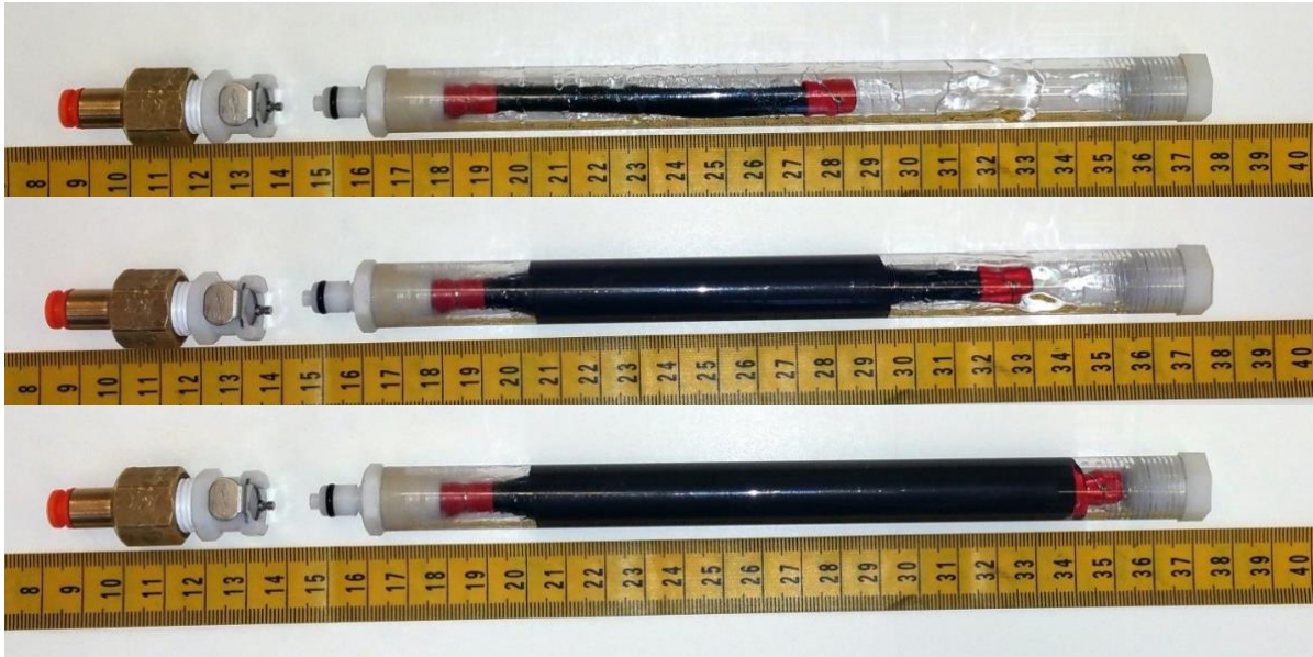
Figure 1.4: Fully assembled custom elastomeric strain energy accumulator as to be used in the recycling pneumatic power scheme. Top image shows uninflated accumulator, middle image shows partially inflated accumulated, bottom image shows fully inflated accumulator. The balloon expands and slides to fill the allowed space by the outer shroud.
