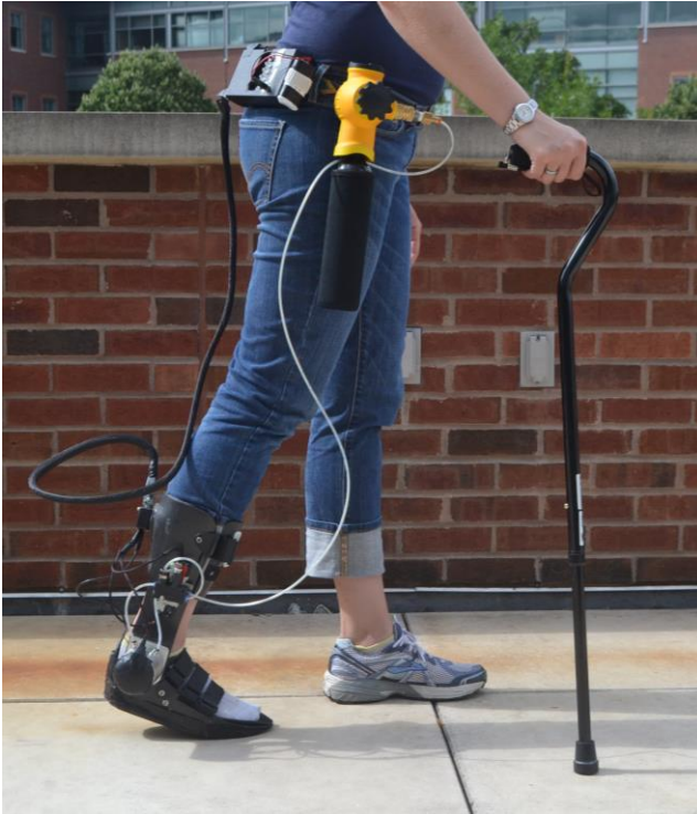
Figure 1.1: Portable Powered Ankle-Foot Orthosis (PPAFO) with waist worn fuel tank and microcontroller.
