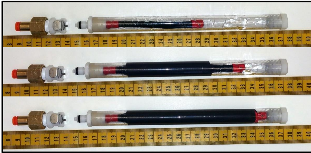
Figure 2.7: Fully assembled custom elastomeric strain energy accumulator used in the recycling circuit. Top image: uninflated accumulator. Middle image: partially inflated accumulator. Bottom image: fully inflated accumulator. The balloon expands and slides to fill the allowed space by the outer shroud.
