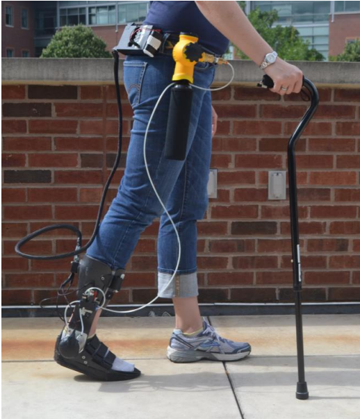
Figure 2.1: Portable Powered Ankle-Foot Orthosis (PPAFO) with waist worn fuel tank and microcontroller.
