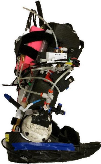
Figure 2.6: PPAFO with accumulator and pressure transducers for longevity testing. All components were attached to the PPAFO for both pneumatic circuits during treadmill testing, so only pneumatic connections needed to be adjusted between trials. For the over-ground walking trials, the pressure transducers on the back and the accumulator were not attached to the PPAFO.
