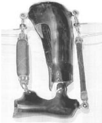
Figure 1.5: Original PAFO design by Ferris et al. 2005 [6]
