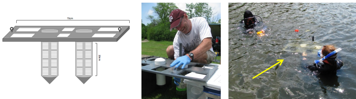
Figure 1: In situ core design and field deployment (credit: Victoria Boyd, UIUC and Peter Van Metre, USGS)
