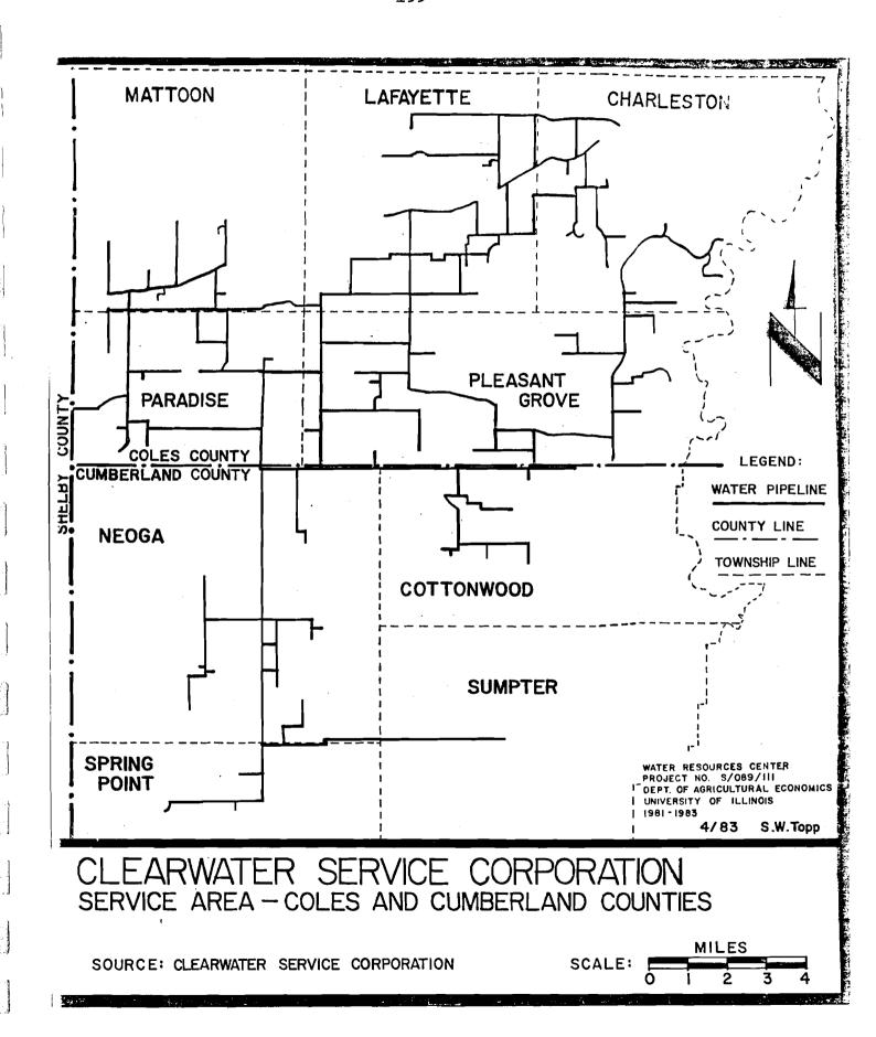
north section connects with the lines that lead into Pleasant Grove Township. The pipeline that heads south splits at the county border, part of it runs due east, paralleling the border, and the part of it extends southward into Cumberland County.
