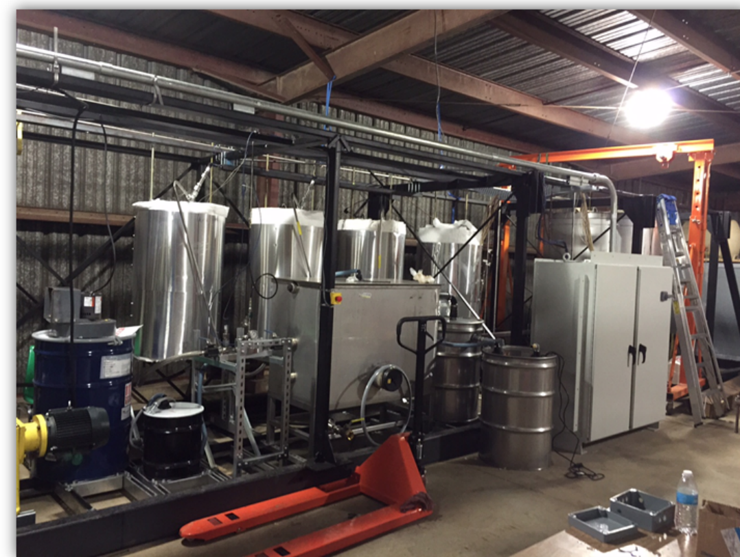
Figure 1 depicts a plug-flow reactor used for hydrothermal liquefaction. (Source: Dr. Yuanhui Zhang)
