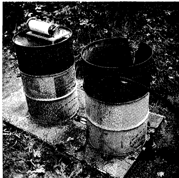
Fig. 20. Stilling and weir barrels were used for surface runoff measurement.
