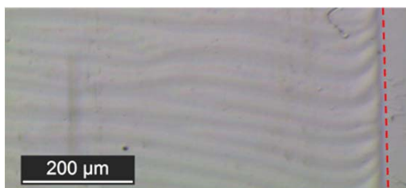
Figure 4.3. The surface of a COC sheet after spin-coating with Novec 1700. The dashed red line separates the coated region (left) from the non-coated region (right).
