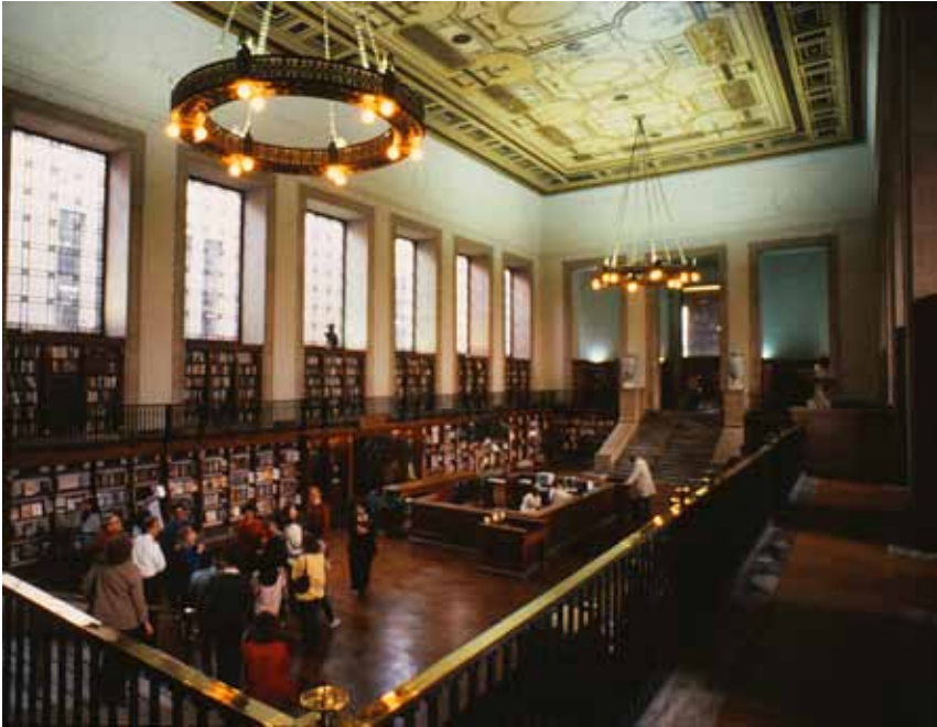
Figure 5. The Indianapolis and Marion County Public Library. The room's chandeliers combine intense uplighting with decorative visible light bulbs. Photograph by Fred Schlipf.
