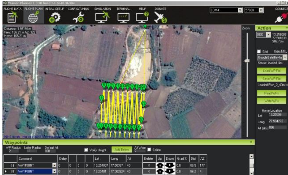
Figure 3.7: Mission Planner Software and flight planning interface. Waypoints can be manually entered in a grid-like pattern and loaded into the Iris for a fully automated flight. Mission Planner can also specify various flight parameters, such as ground speed, altitude, takeoff and landing locations, and can task the Iris to perform 360 panoramic turns.
