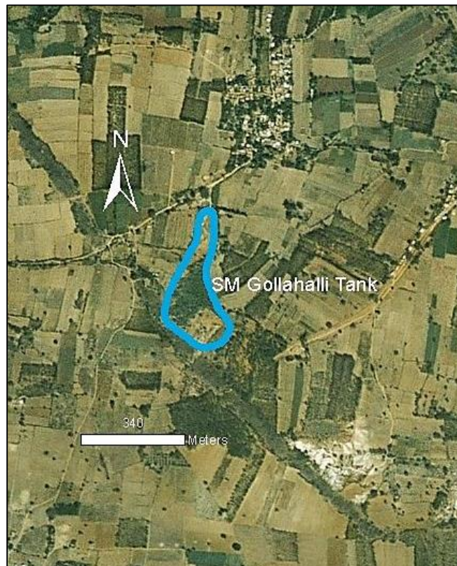
Figure 3.5: Boundary of SM Gollahalli tank surveyed with a UAV and USV, highlighted in blue. The area surveyed aerially was 44,000 m 2 . The middle portion of the tank had dense tree cover; however, this area was generally very flat and important topography changes were not missed with the UAV.
