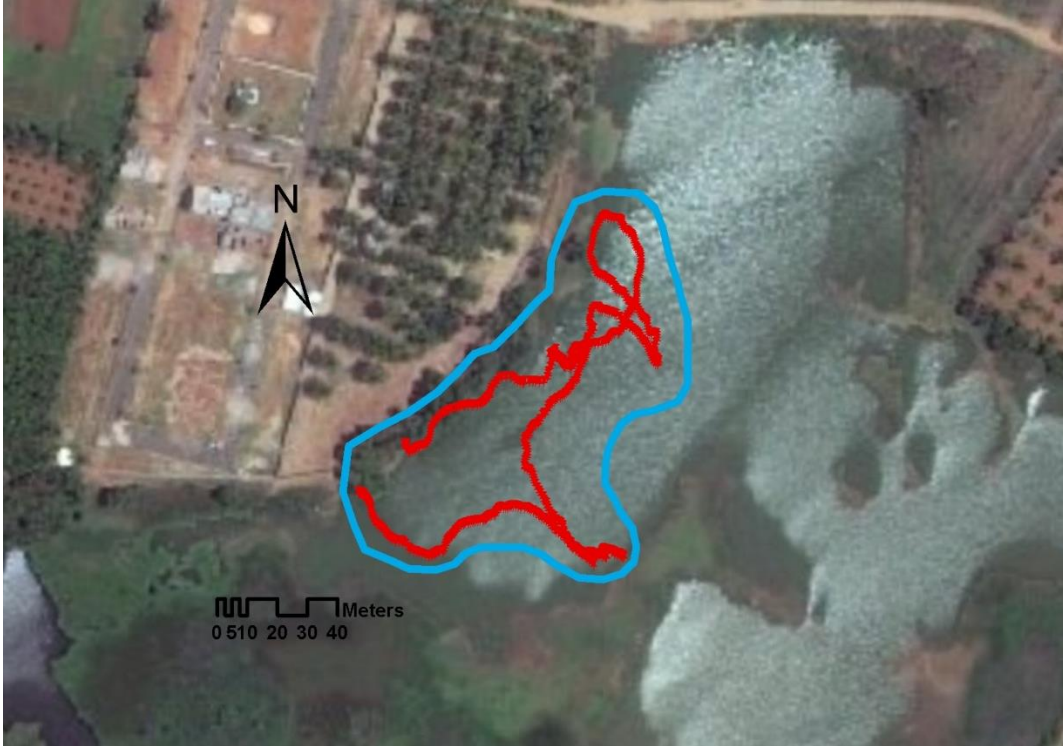
Figure4.3: Visualization of GPS tagged bathymetric photos at Nelamangala Lake. Each red dot represents a photo taken of the HawkEye depth finder reading; an example is shown below in Figure 4.4.
