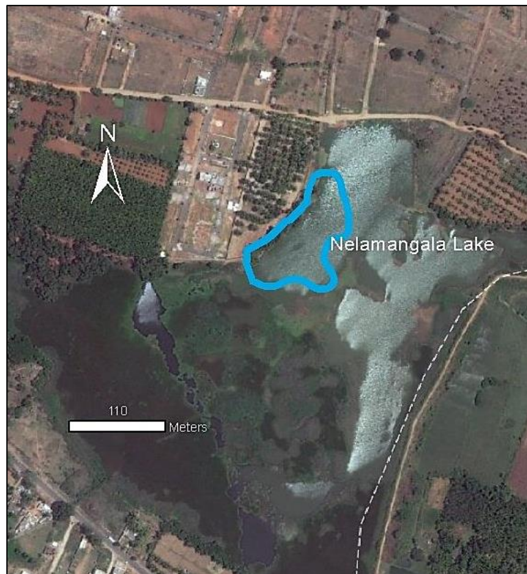
Figure 3.4: Location of Nelamangala Lake. The outline in blue refers to the boundary of the portion of the lake surveyed with a USV, which measured approximately 8,200 m 2 . A majority of the west side of the lake was heavily covered in vegetation and was incapable of being navigated through with the USV.
