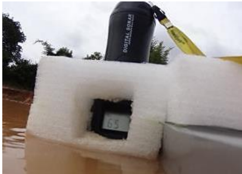
Figure 4.9: Sample image of a HawkEye Depth reading at SM Gollahalli tank. The depth reading for each image was manually recorded, stored as a .csv along with extracted GPS information, and imported into GIS for surface interpolation.
