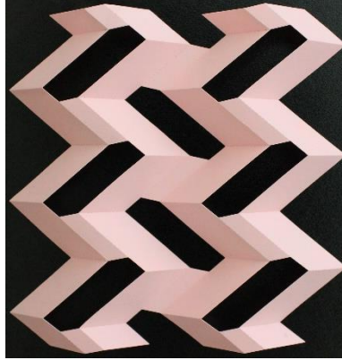
Figure 5.7: A developable ZCH pattern with augmented bonding areas.
