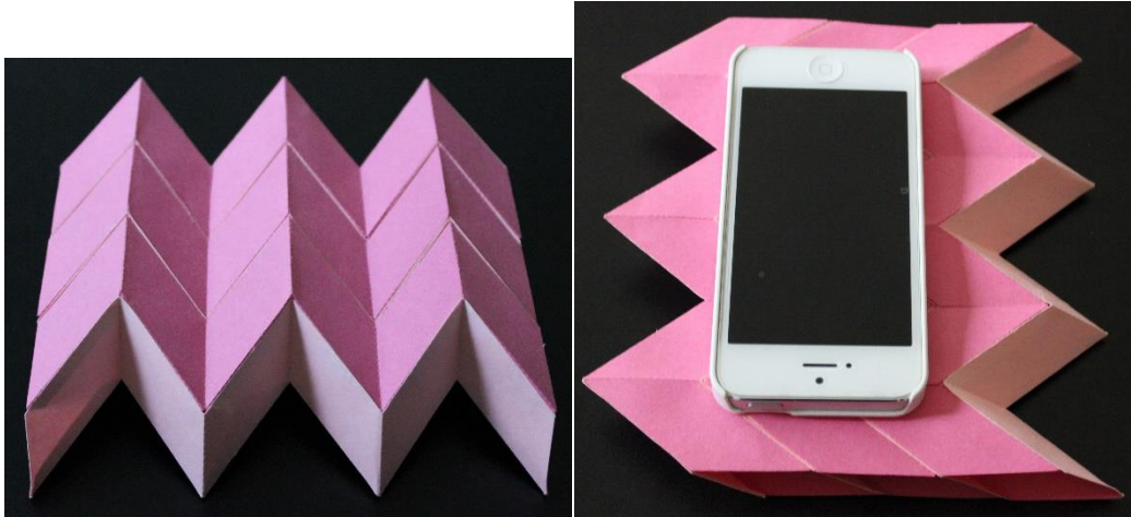
Figure 3.22: A side-by-side assembly of the tubes shown in the figure above. The structure is flat-foldable in one direction and can carry vertical loads in its deployed configuration.
