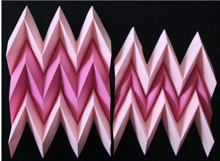
Figure 3.20: Non-developable zigzag-base patterns constructed from Miura-ori cells with identical kinematics and different heights of the unit cells (the rule is similar to that used in the stacking, but the cells possessing different heights are connected side-by-side instead of stacking).
