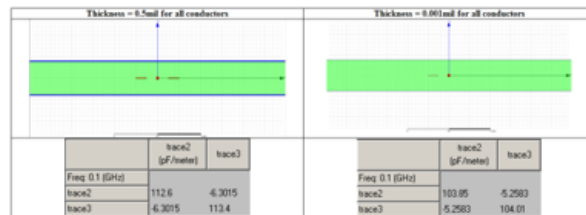
Figure 3.7: Cross-sectional view of the multi-conductor stripline models with 2 conductors at two different thicknesses
