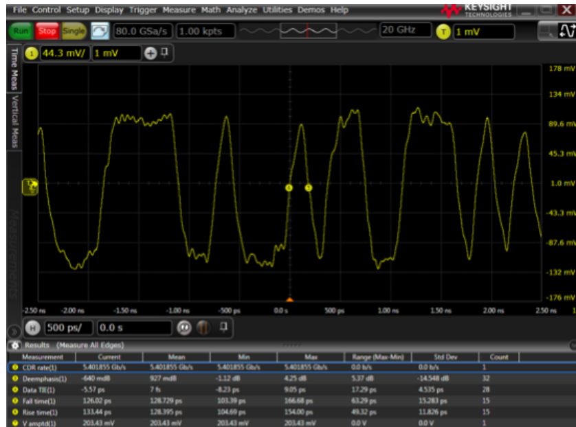
Figure 4.13: Waveform with 20 GHz BW limitation
