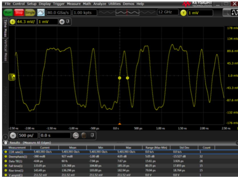
Figure 4.14: Waveform with 12 GHz BW limitation
