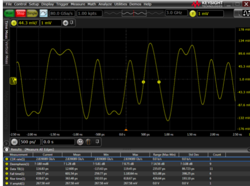
Figure 4.16: Waveform with 3 GHz BW limitation
