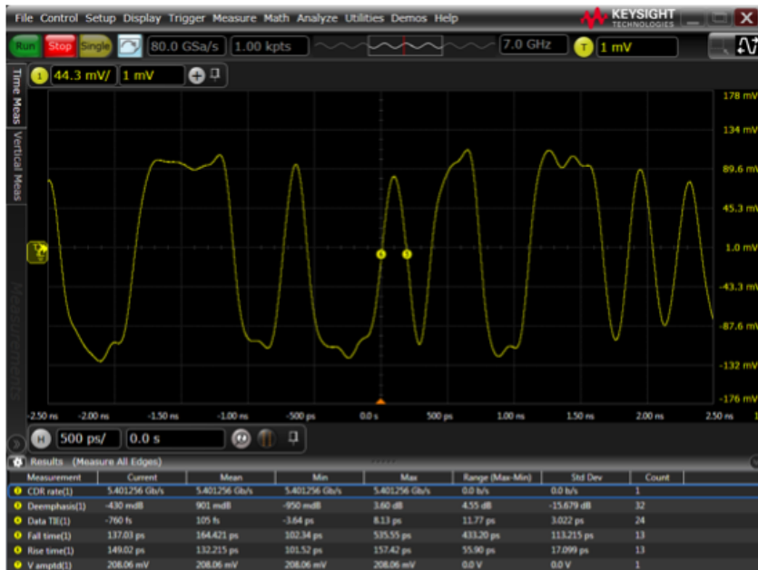
Figure 4.15: Waveform with 7 GHz BW limitation
