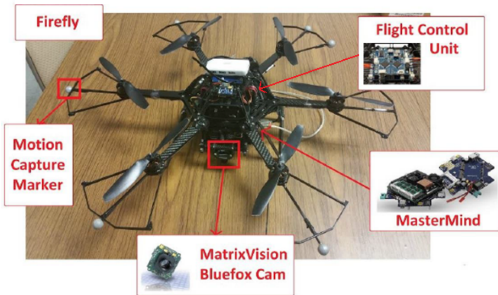
Figure 3.6: Experimental setup of the AscTec Firefly equipped with the Bluefox camera, MasterMind board, flight control unit, and motion capture markers.
