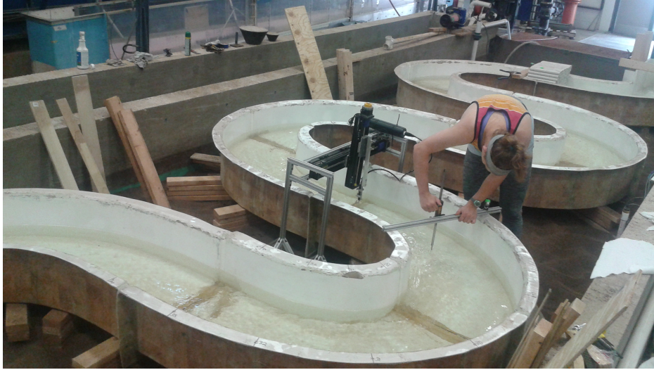
Figure 4.1: Experimental flume and ADV
