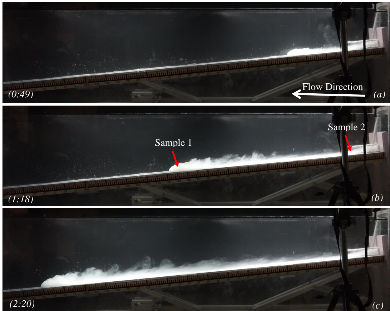
Figure 12 - These figures (a through d) depict the evolution of a typical hyperpycnal flow in the tank. Locations of samples taken during the run are marked on the figure, as well as the time elapsed since inflow began. Figure 10(a) shows the initial density current. Figure 10(b) shows the same hyperpycnal flow when the front has moved farther down the sloping platform. Figure 10(c) shows the front and flow behind as it approaches the end of the sloping platform, and features shedding vortices. Figure 10(d) shows the flow after the front has passed out of the Shelf Tank.
