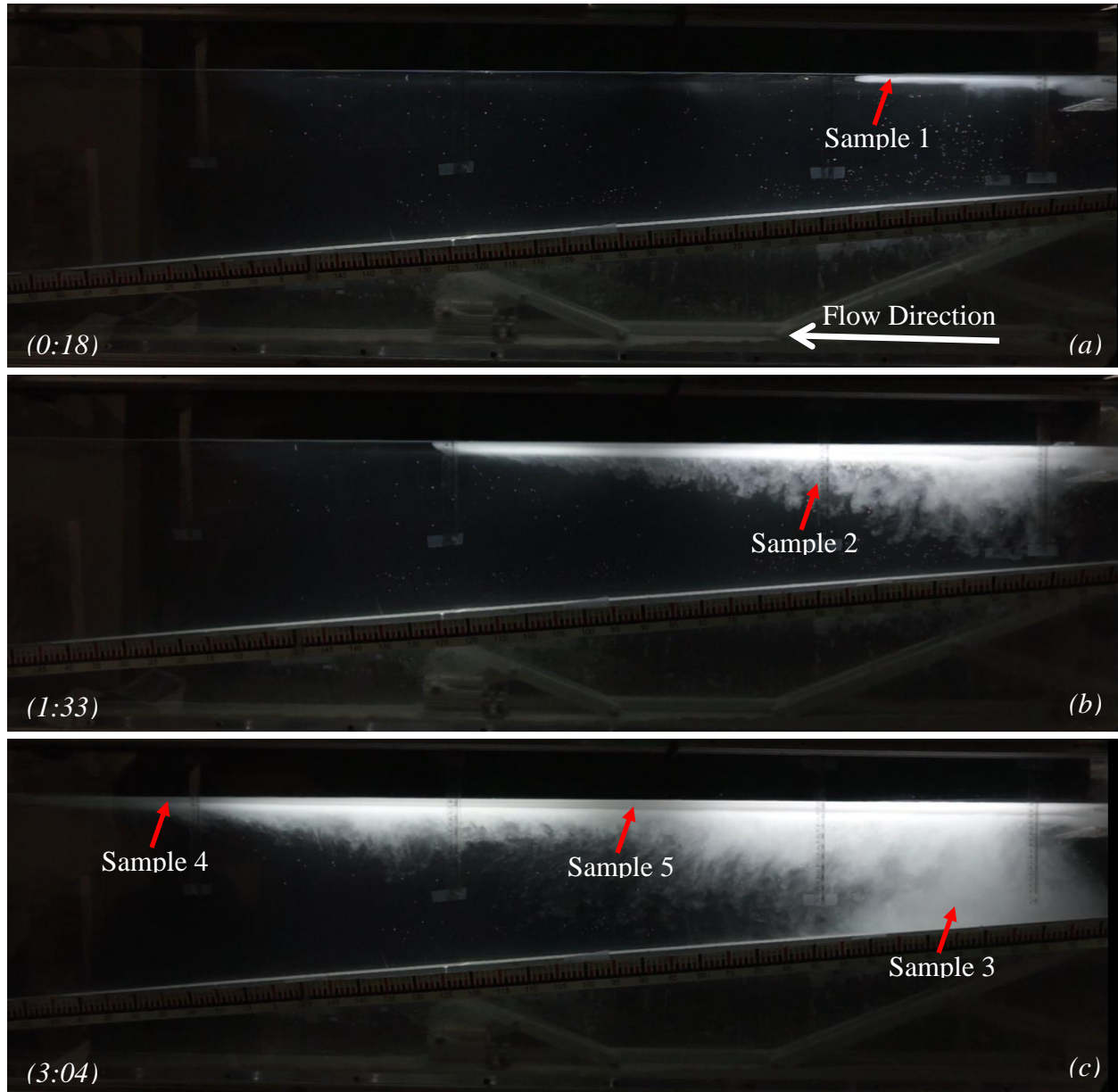
Figure 8 - These figures ( a through e ) depict the evolution of a typical hypopycnal flow in the tank. Locations of samples taken during the experiment are marked on the images, as well as the time from the beginning of inflow. Figure 6(a) shows the initial hypopycnal plume, before fingering begins. Figure 6(b) shows the fingers as the plume moves downstream. Figure 6(c) shows the incipient hyperpycnal flow as the fingers reach the bed and accumulate. Figure 6(d) shows the hyperpycnal and hypopycnal flows coexisting as both move downstream. Figure 6(e) shows the hyperpycnal plume as it begins to separate from the bed to form an interflow.
