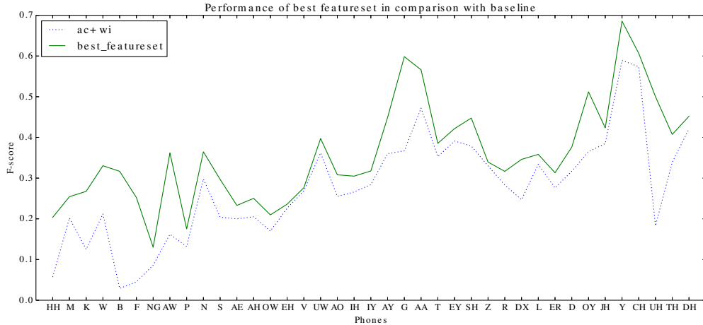
Figure 5.10: Comparison between the best feature subset and ac+wi baseline on the training set using LinearSVC and the Auto-Weighting approach, where the f1_score is averaged over all 10 folds. The sequence of phones is sorted by the percentage of pronunciation errors.
