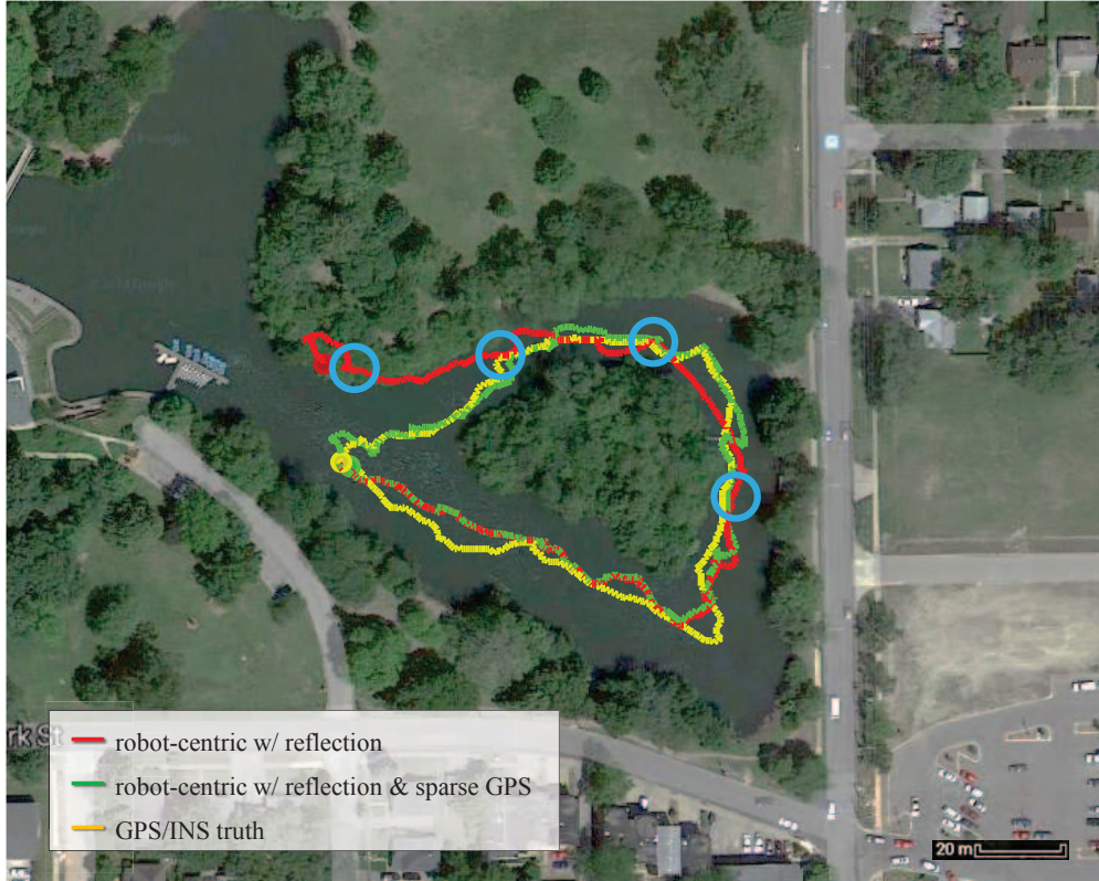
Figure 3.14: The experimental results show that a short sequences of badly estimated poses (blue circles) can cause the pose estimates to drift (red). The localization result that is obtained when GPS data are provided as measurements to the smoothing filter around these points is also shown (green).
