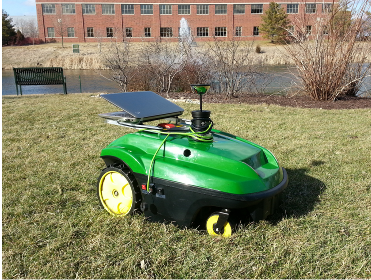
Figure 4.1: Our autonomous mower modified with an omnidirectional camera and an IMU for experiments.
