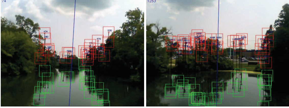
Figure 3.4: The results of reflection feature detection with the reflection matching Algorithm 1. The real objects (red boxes), the corresponding reflections (green boxes), the matching slope \theta_i (black lines), and the reference slope \theta_0 (blue line in the middle of the image) are shown.
