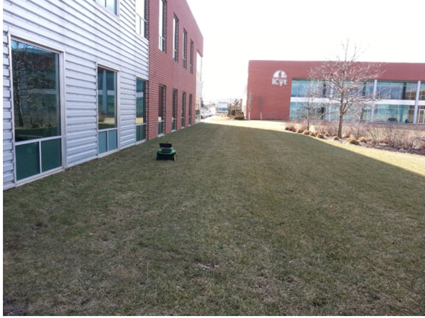
Figure 4.9: Our autonomous mower following a boundary set-up in the backyard of our research building for the map estimation and the boundary teaching.
