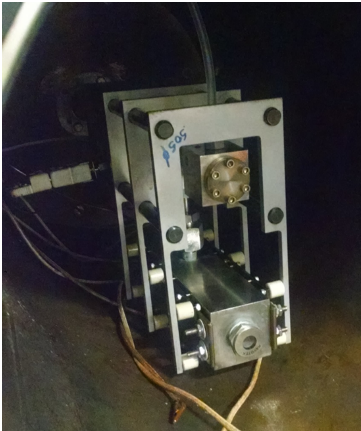
Figure 4.7: Second-generation extraction chamber. It includes new 500 W heating strips to ensure the necessary temperatures for a toluene-containing fluid can be reached. Also visible are the new sight glass and a steel-jacketed thermocouple extending into the body of the chamber to allow direct monitoring of the supercritical fluid temperature.
