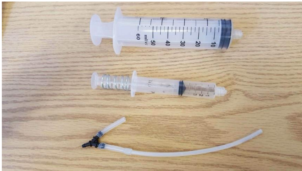
Figure 36: 60ml and 10 ml syringes with wye valve and pneumatic tubing
