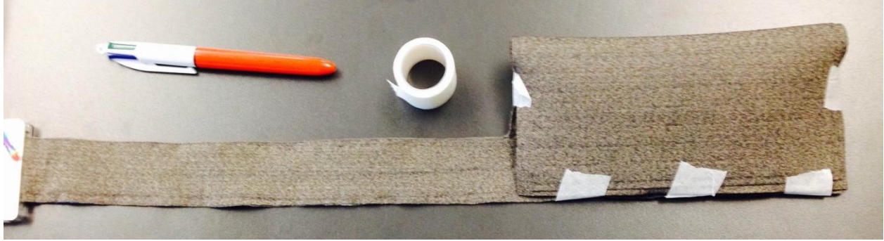
Figure 16: Novel Pliance sensor folded in half and taped.
