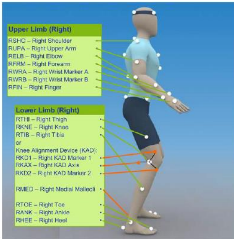
Figure 12: PIG marker placement (side)
