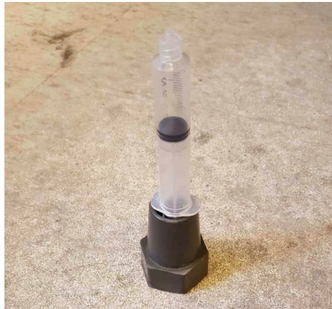
Figure 33: Pneumatic cylinder (10 ml total, 2.4 ml effective volume) inserted into a crutch tip bumper
