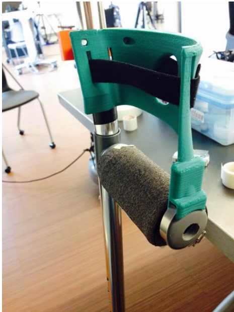
Figure 17: Novel Pliance sensor wrapped around handle with orthotic.
