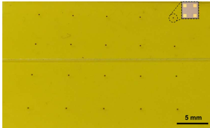
Figure 74: Image of a sparse array of silicon chip printed onto an acceptor substrate using a collect and place printing more.
