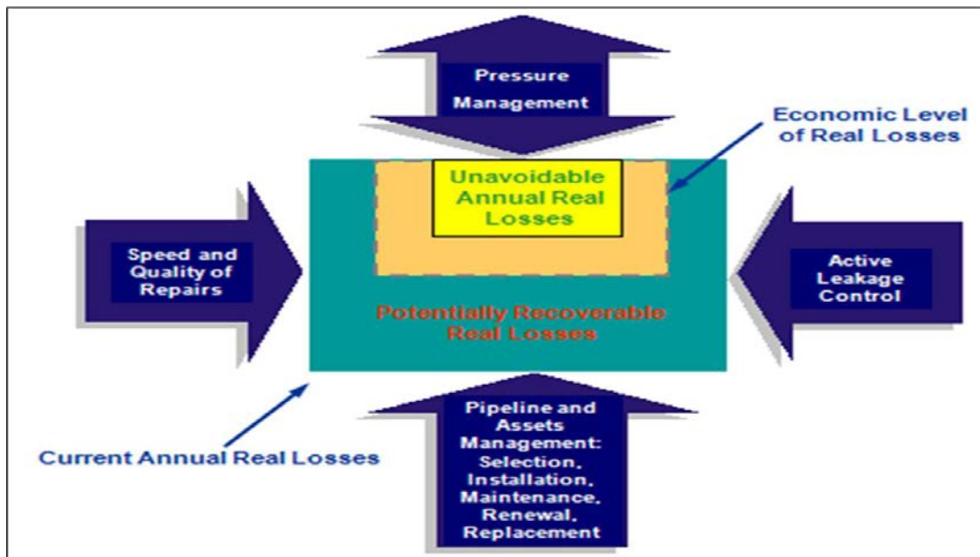
Figure 1.1 Methods to reduce leakage (Pearson 1995).
