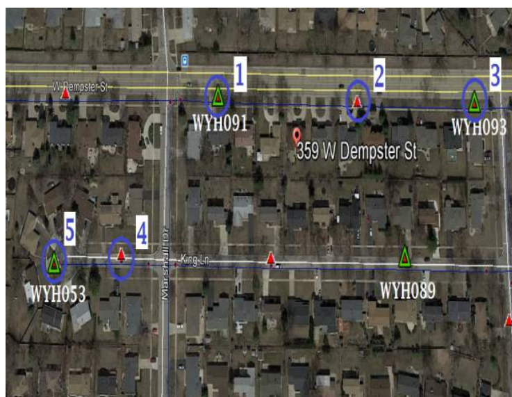
Figure 3.8 Acoustic loggers near 359 Dempster Street leak.
