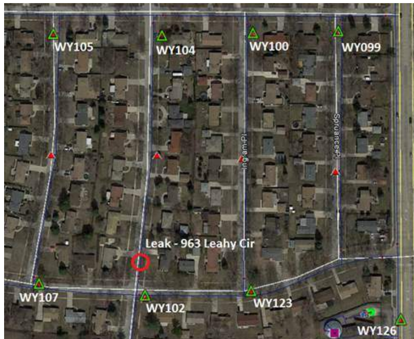
Figure 3.17 Acoustic monitors near 963 Leahy Circle leak.
