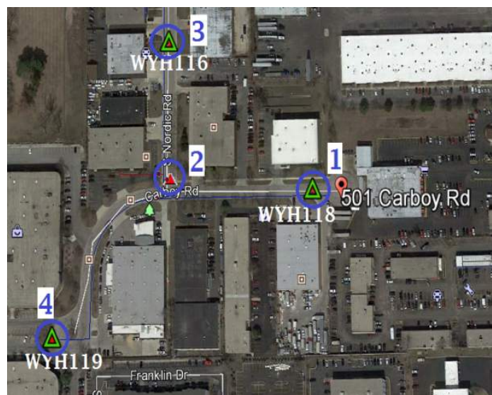
Figure 3.11 Location of acoustic monitors near 501 Carboy leak.
