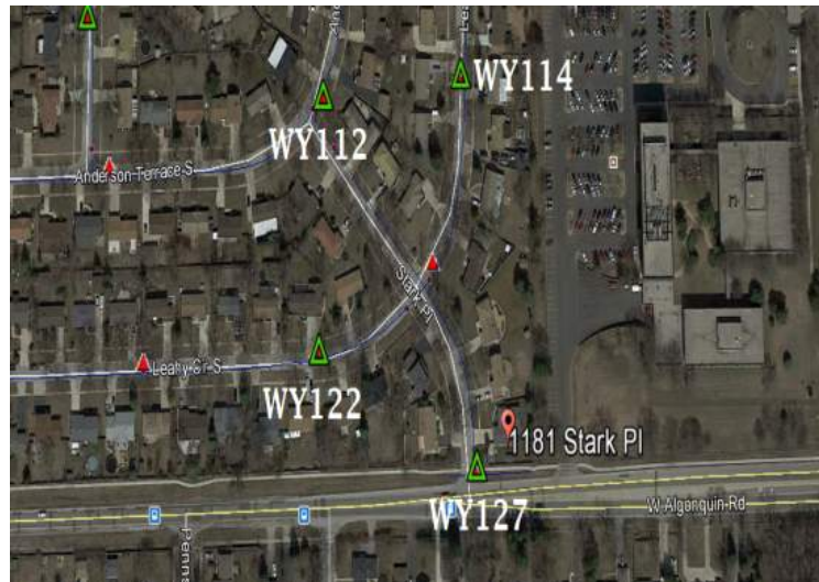
Figure 3.14 Locations of acoustic monitors near 1181 Stark Place leak.
