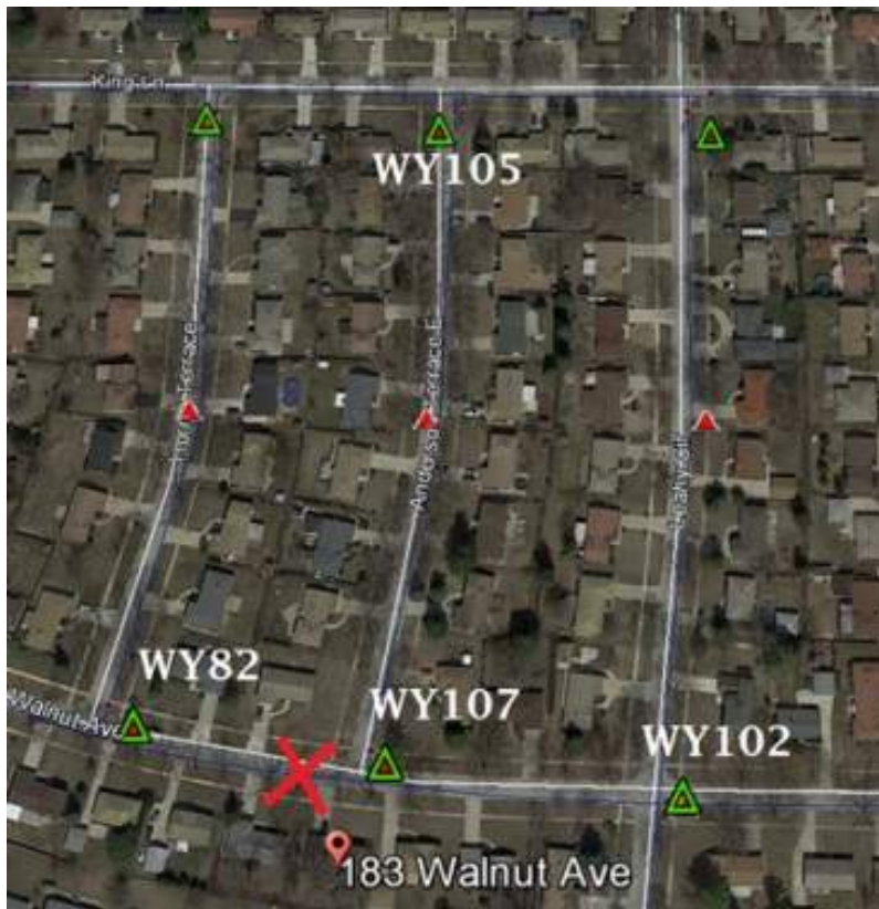
Figure 3.16 Acoustic monitors near 183 West Walnut leak.
