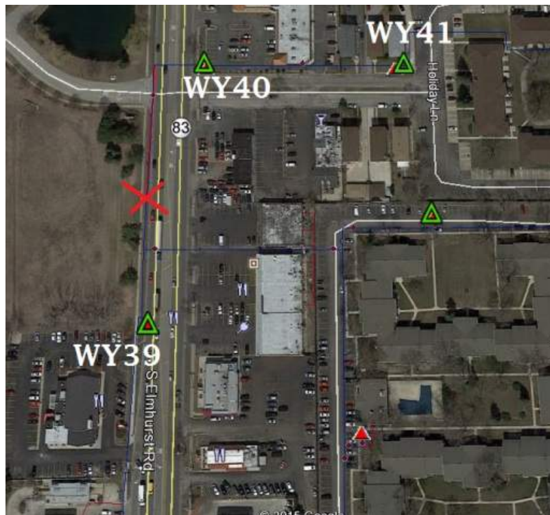
Figure 3.15 Acoustic monitors near 1101 Elmhurst leak.
