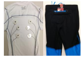
Figure 2. Compression suit with EMG sensors and TESSEL.
