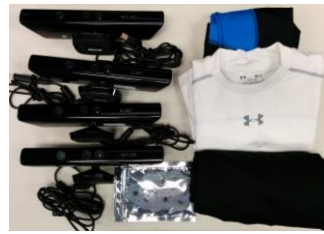
Figure 1. CyPhy kit: Kinects, compression suit, mat, and extra electrodes.
