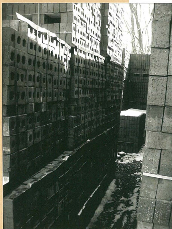
Figure 1 Five thousand full-size bricks made in commercial-scale run using a beehive kiln.
