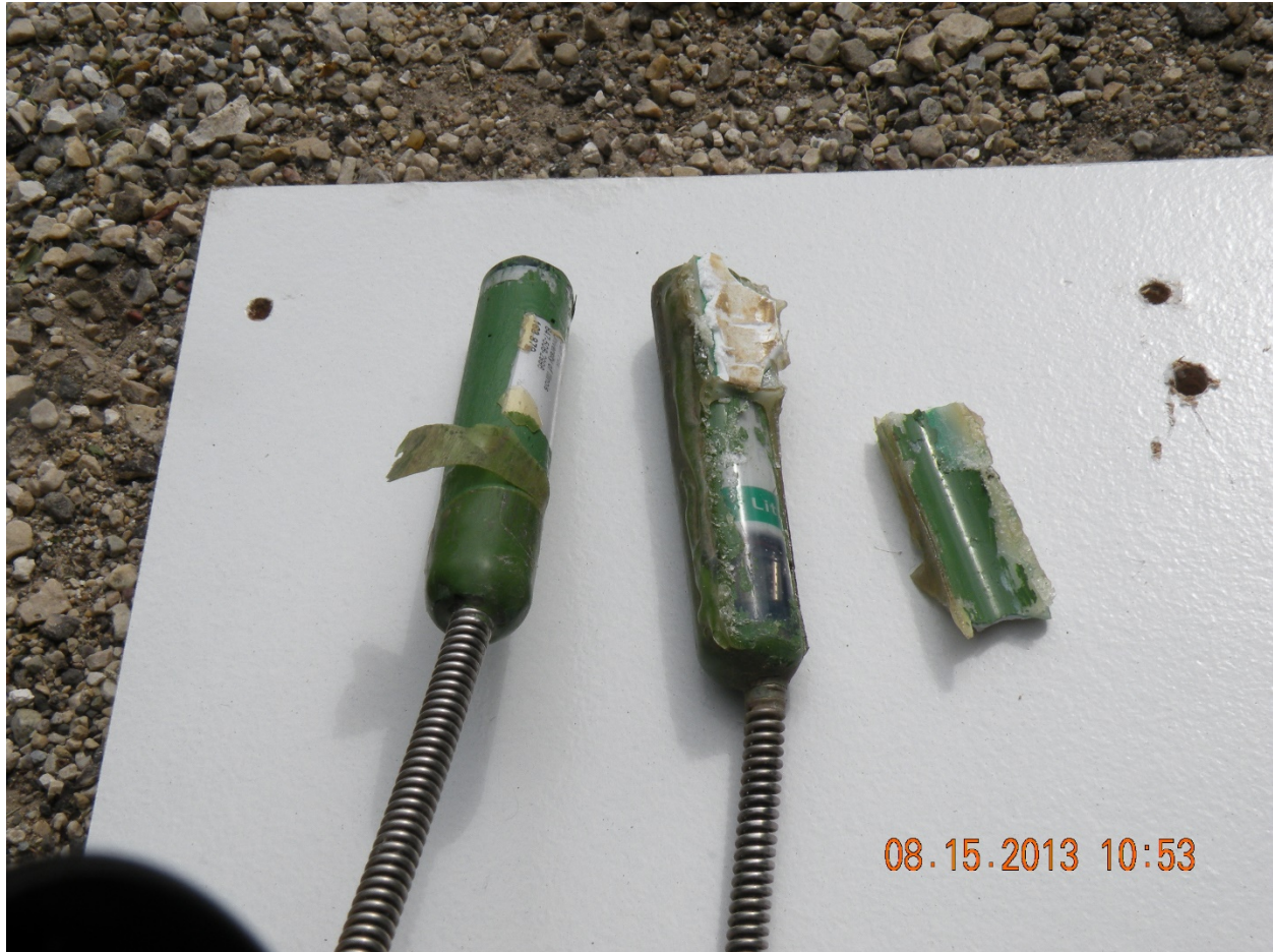
Figure 8: Two examples of transmitter failure via detachment from leg-bands. The transmitter on the left was deployed on 6/21/2012 and was recovered on 5/13/2013. Note the peeling of the outer coating of the transmitter, remnants of which visibly remained on the bird's leg band. The transmitter on the right was deployed for a comparable length of time but was recovered prior to detachment (note the remnants of the old bands that remained attached to the epoxy). This example demonstrates how the colored coating underlying the clear coating cracked, which often resulted in separation from the epoxy used to attach transmitters to bands (i.e. epoxy was frequently observed on birds' leg bands post transmitter detachment, similar to the fragment on the right). The manufacturer refused to allow us to speak with their engineers to resolve these problems but confirmed that none of the units should have been assembled with these two outer coatings.
