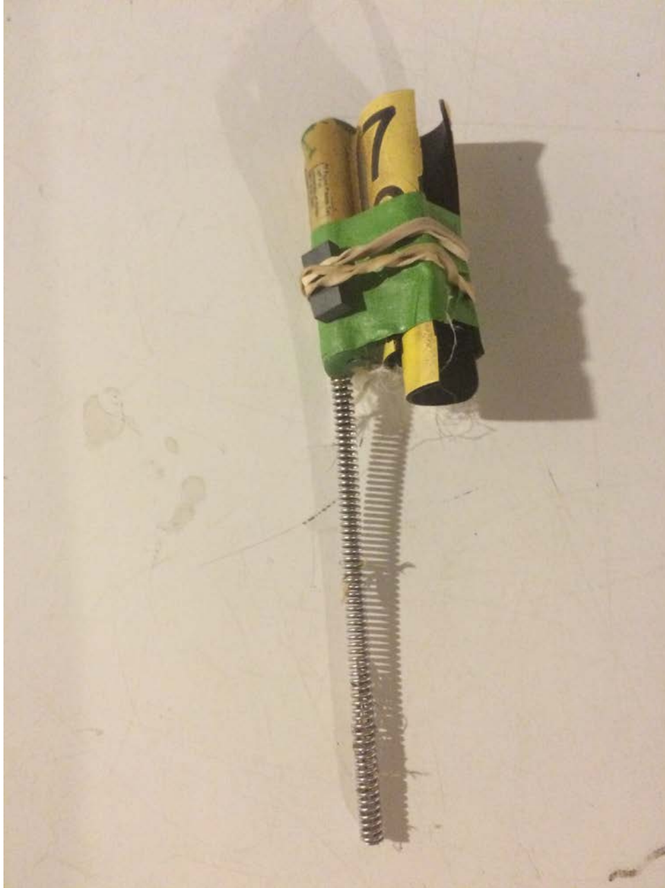
Figure 10: This transmitter was deployed on 7/27/2012 and removed from the bird during a recapture on 7/3/2014. Note that the antenna had completely fallen off and only the spring remained, resulting in a non-functional transmitter. This mode of failure was noted to begin occurring within less than two years post-deployment and appeared to be systemic. The manufacturer claimed that the antenna was not an integral component of a functional transmitter.
