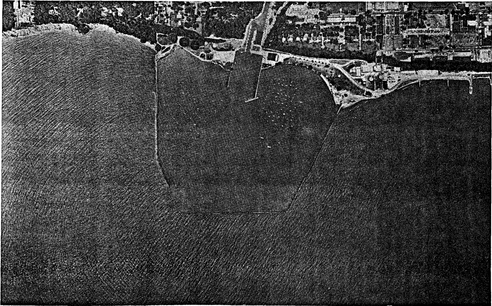
Fig. 16 - Great Lakes Naval Training Center harbor at near record high water levels in late June 1974. Note the submerged condition of the north and south fillets. Strong winds are from the southeast causing a wind shadow inside the north jetty as well as near the shoreward end of the south jetty. Wind streaks can be seen across the harbor. Waves are reflected from the end of the east jetty whereas waves are refracted into the west side of the harbor mouth and around the south jetty to the southern shore.
