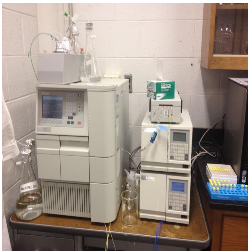
Figure E.4 Waters Alliance e2695 HPLC system with Waters 2489 UV/Visible Detector.
