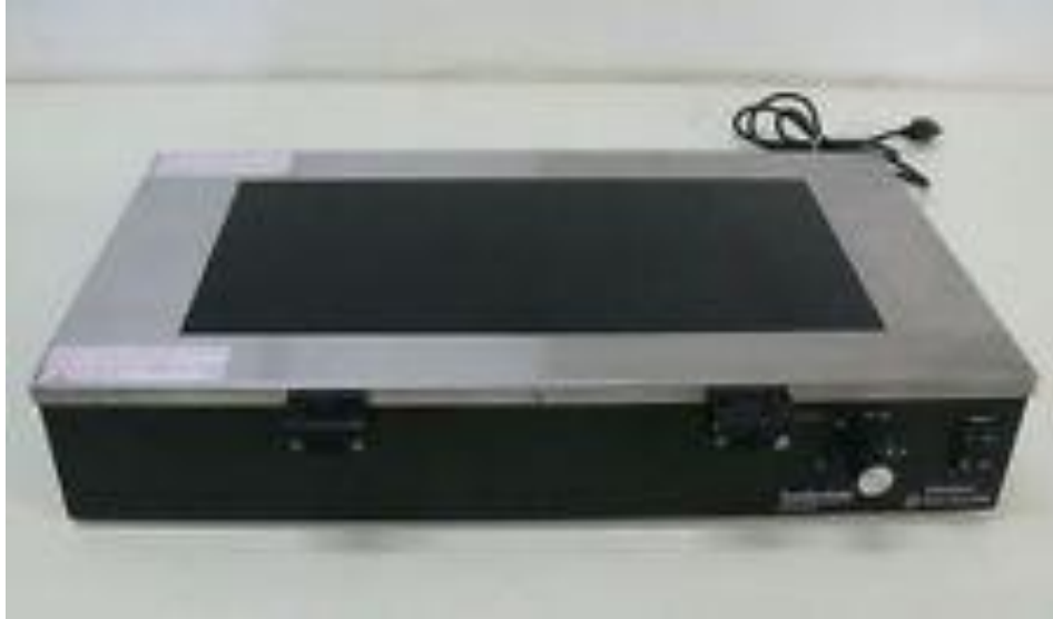
Figure E.5 FisherBiotech™ Ultraviolet Transilluminator (model FBTIV-614).
