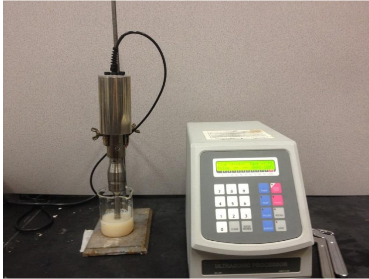
Figure E.1 VC 750 ultrasonic processor (20 kHz) and ultrasonic probe (13 mm diameter).
