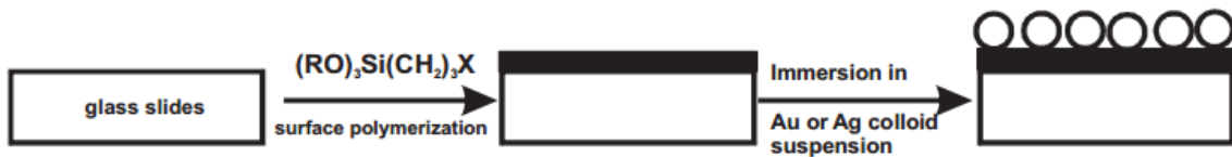
Figure 2.2 Example of chemical attachment method for self-assembly MNPs on glass slide. X can be CN, NH 2 , 2-pyridyl, P(C 6 H 5 ) 2 , or SH; R=CH 3 or CH 2 CH 3 (adapted from [1].)
