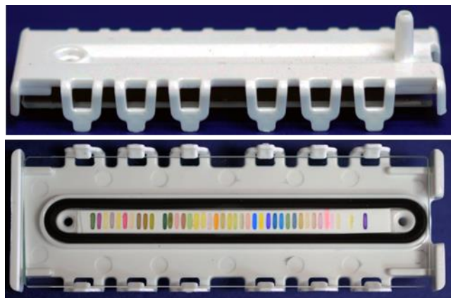
Figure 3.2 Photographs of the cartridge and a colorimetric sensor array showing side and array views. The sensor array shown here has 40 sensor elements at 1.2 mm center-to-center spacing and represents typical printing quality.
