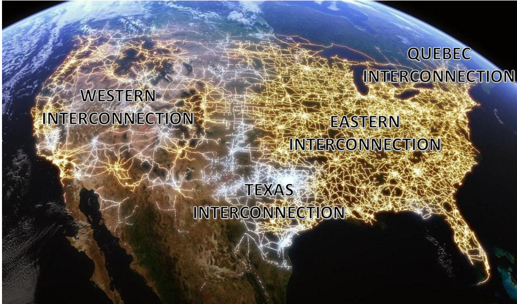
Figure 1.1: An aerial illustration of the geo-spatial structure of the North American electric grid. Transmission lines at voltage levels higher than 160 kV have been artificially colored. Adapted from [6].
